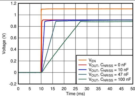
$V_{IN} = 1.2\text{ V}$ ,  $V_{OUT} = 0.9\text{ V}$ ,  $V_{BIAS} = 5.0\text{ V}$ ,  $I_{OUT} = 4\text{ A}$ ,  $C_{OUT} = 47\text{ }\mu\text{F} \parallel 10\text{ }\mu\text{F} \parallel 10\text{ }\mu\text{F}$ ,  $C_{FF} = 10\text{ nF}$
