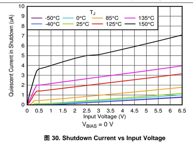
图 30. Shutdown Current vs Input Voltage
