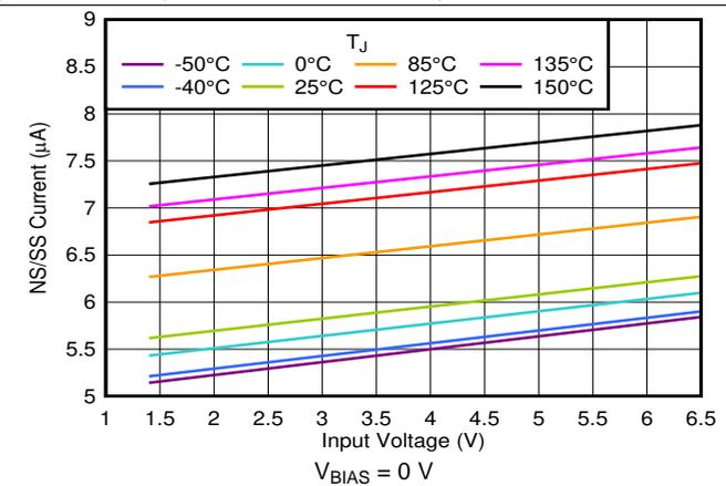
图 32. NR/SS Current vs Input Voltage and Temperature
