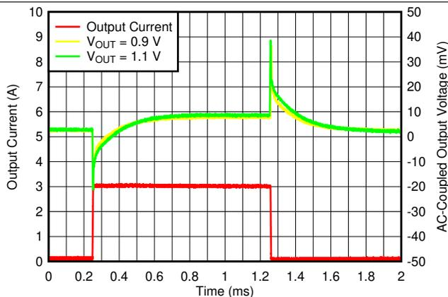
$I_{OUT, DC} = 100\text{ mA}$ ,  $C_{OUT} = 47\text{ }\mu\text{F} \parallel 10\text{ }\mu\text{F} \parallel 10\text{ }\mu\text{F}$ ,  $C_{NR/SS} = C_{FF} = 10\text{ nF}$ , slew rate =  $1\text{ A}/\mu\text{s}$
