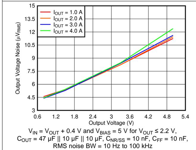
图 9. Output Voltage Noise vs Output Voltage
