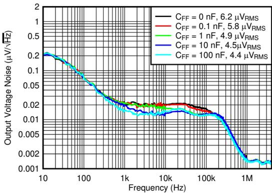
$V_{IN} = V_{OUT} + 0.4\text{ V}$ ,  $V_{BIAS} = 5\text{ V}$ ,  $I_{OUT} = 4\text{ A}$ , sequencing with a DC/DC converter and PG,  $C_{OUT} = 47\text{ }\mu\text{F} \parallel 10\text{ }\mu\text{F} \parallel 10\text{ }\mu\text{F}$ ,  $C_{NR/SS} = 10\text{ nF}$ , RMS noise BW = 10 Hz to 100 kHz
