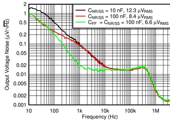
$V_{IN} = 5.6\text{ V}$ ,  $I_{OUT} = 4\text{ A}$ ,  $C_{OUT} = 47\text{ }\mu\text{F} \parallel 10\text{ }\mu\text{F} \parallel 10\text{ }\mu\text{F}$ ,  $C_{FF} = 10\text{ nF}$ , RMS noise BW = 10 Hz to 100 kHz
