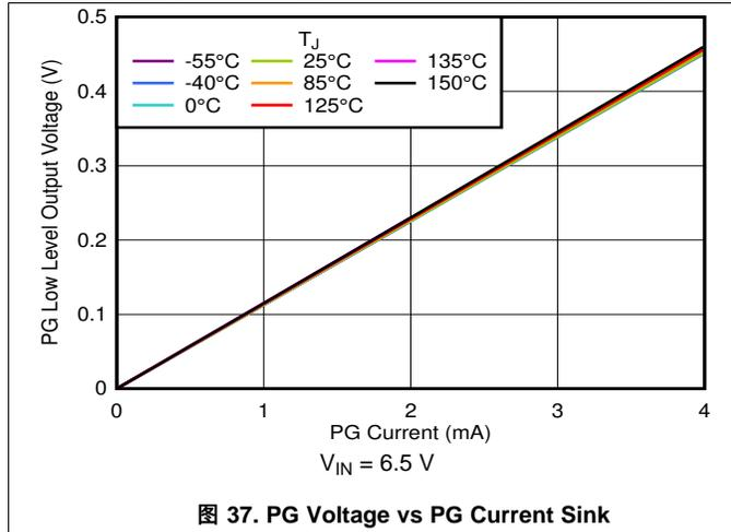
图 37. PG Voltage vs PG Current Sink
