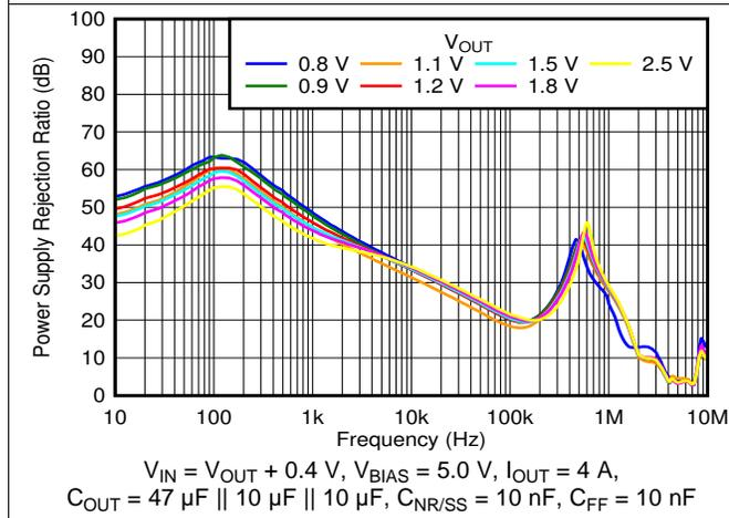
图 5. PSRR vs Frequency and  $V_{OUT}$  With Bias
