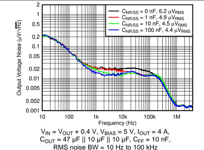
图 12. Output Noise vs Frequency and  $C_{NR/SS}$
