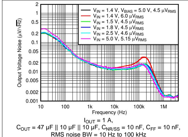
图 11. Output Noise vs Frequency and Input Voltage
