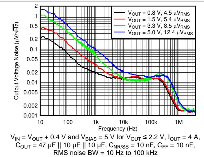
图 10. Output Noise vs Frequency and  $V_{OUT}$
