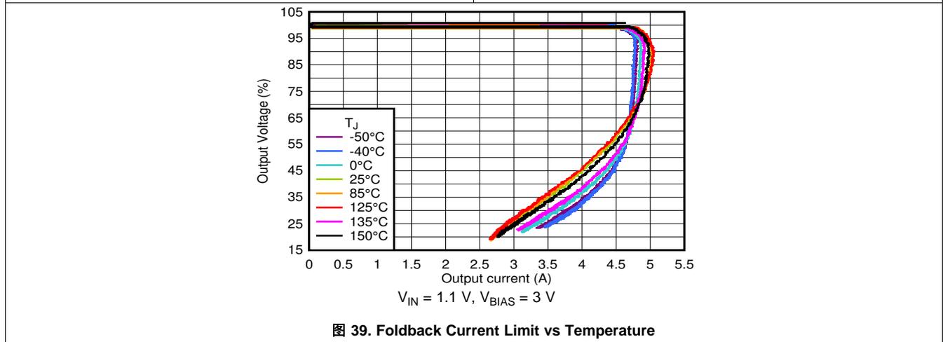
图 39. Foldback Current Limit vs Temperature
