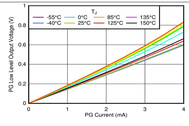
图 36. PG Voltage vs PG Current Sink
