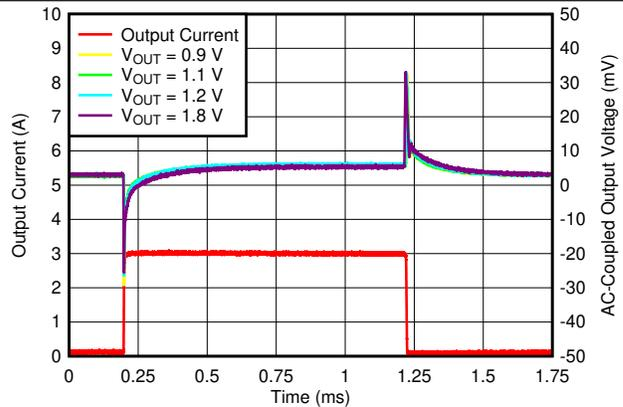
$V_{IN} = V_{OUT} + 0.3\text{ V}$ ,  $V_{BIAS} = 5\text{ V}$ ,  $I_{OUT, DC} = 100\text{ mA}$ , slew rate =  $1\text{ A}/\mu\text{s}$ ,  $C_{NR/SS} = C_{FF} = 10\text{ nF}$ ,  $C_{OUT} = 47\text{ }\mu\text{F} \parallel 10\text{ }\mu\text{F} \parallel 10\text{ }\mu\text{F}$
