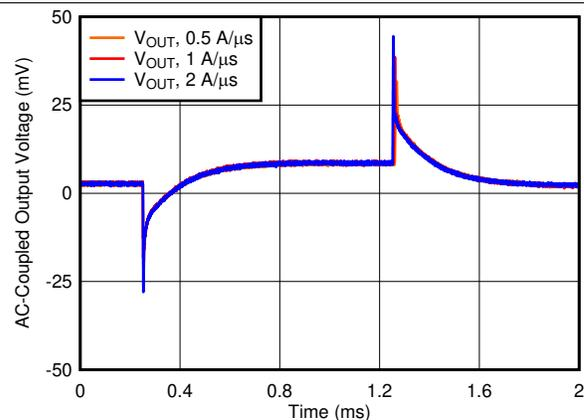
$V_{OUT} = 5\text{ V}$ ,  $I_{OUT, DC} = 100\text{ mA}$ ,  $I_{OUT} = 100\text{ mA}$  to  $4\text{ A}$ ,  $C_{OUT} = 47\text{ }\mu\text{F} \parallel 10\text{ }\mu\text{F} \parallel 10\text{ }\mu\text{F}$ ,  $C_{NR/SS} = C_{FF} = 10\text{ nF}$
