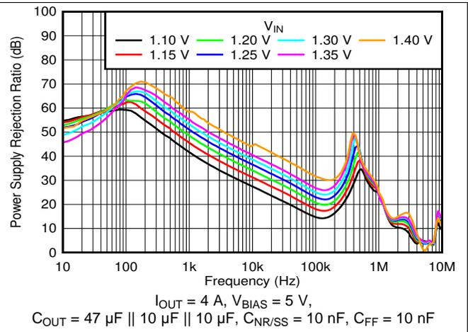
图 2. PSRR vs Frequency and  $V_{IN}$  With Bias
