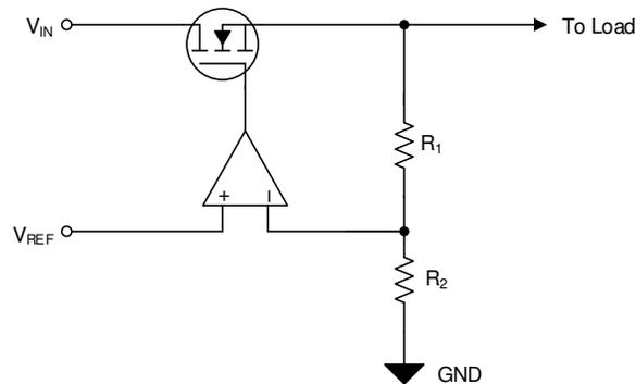
NOTE:  $V_{OUT} = V_{REF} \times (1 + R_1 / R_2)$ .
