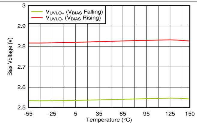
图 34.  $V_{BIAS}$  UVLO vs Temperature
