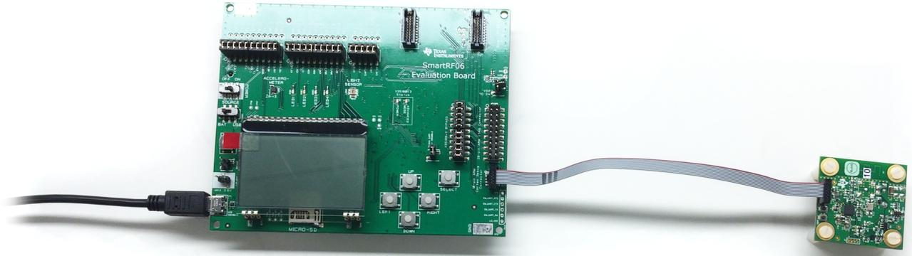
**图 10. Connection of SmartRF06 Evaluation Board and TI Designs Hardware for Programming/Debugging**
