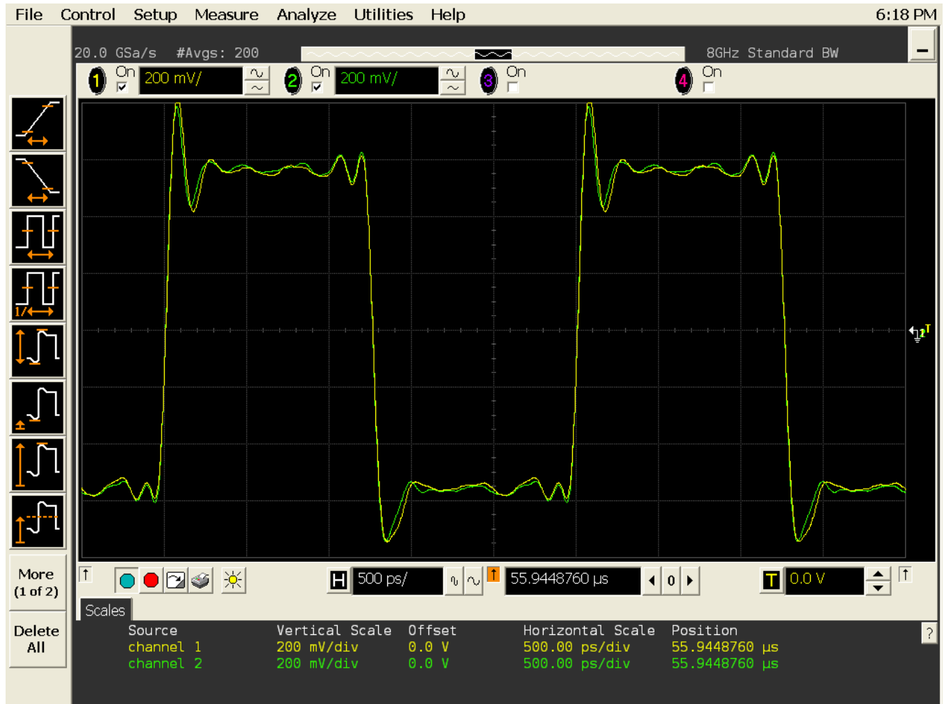
图 7. Non-Critical SYNC Example After SYNC Pulse
