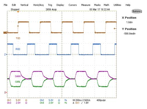
图 8. CAN Waveforms With 5 Mbps of Data
