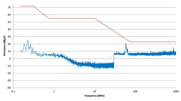
图 15. Noise Floor Measurement of Conducted Emissions Test Equipment
