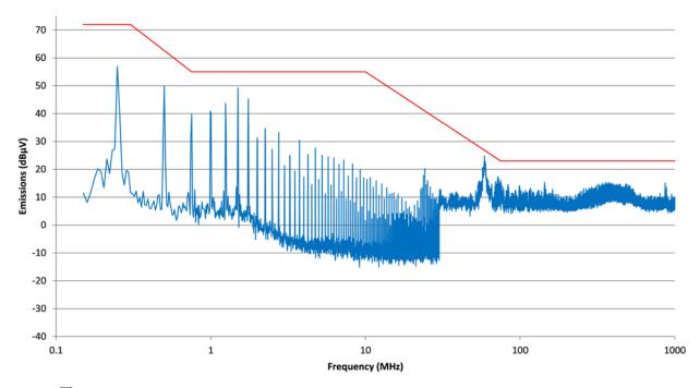
图 16. Common-Mode Choke Measurement of Conducted Emissions Test Equipment
