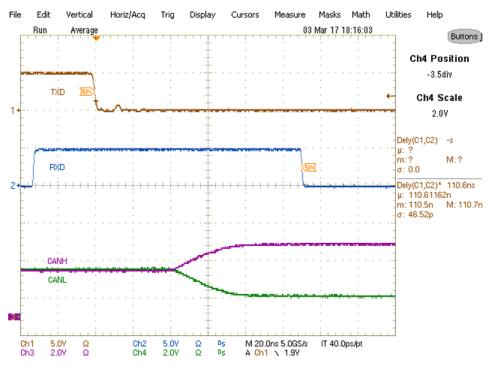
图 12. T<sub>PROP(LOOP1)</sub> Delay Measured With 5 Mbps of Data
