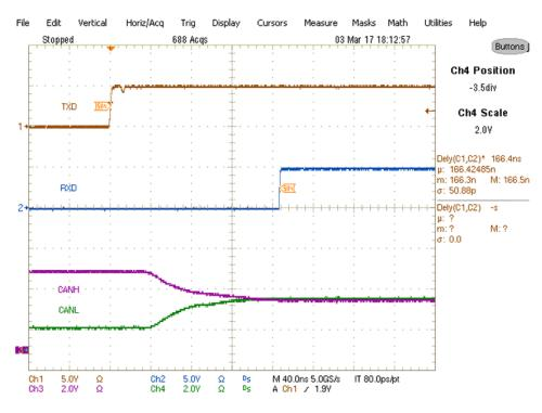
图 11. T PROP(LOOP2) Delay Measured With 1 Mbps of Data
