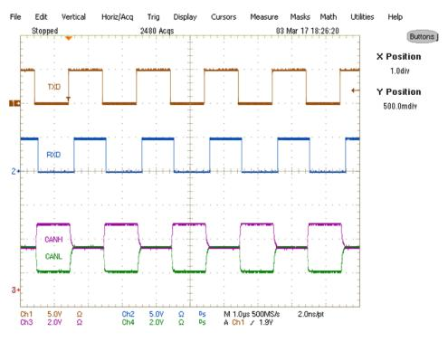
图 7. CAN Waveforms With 1 Mbps of Data
