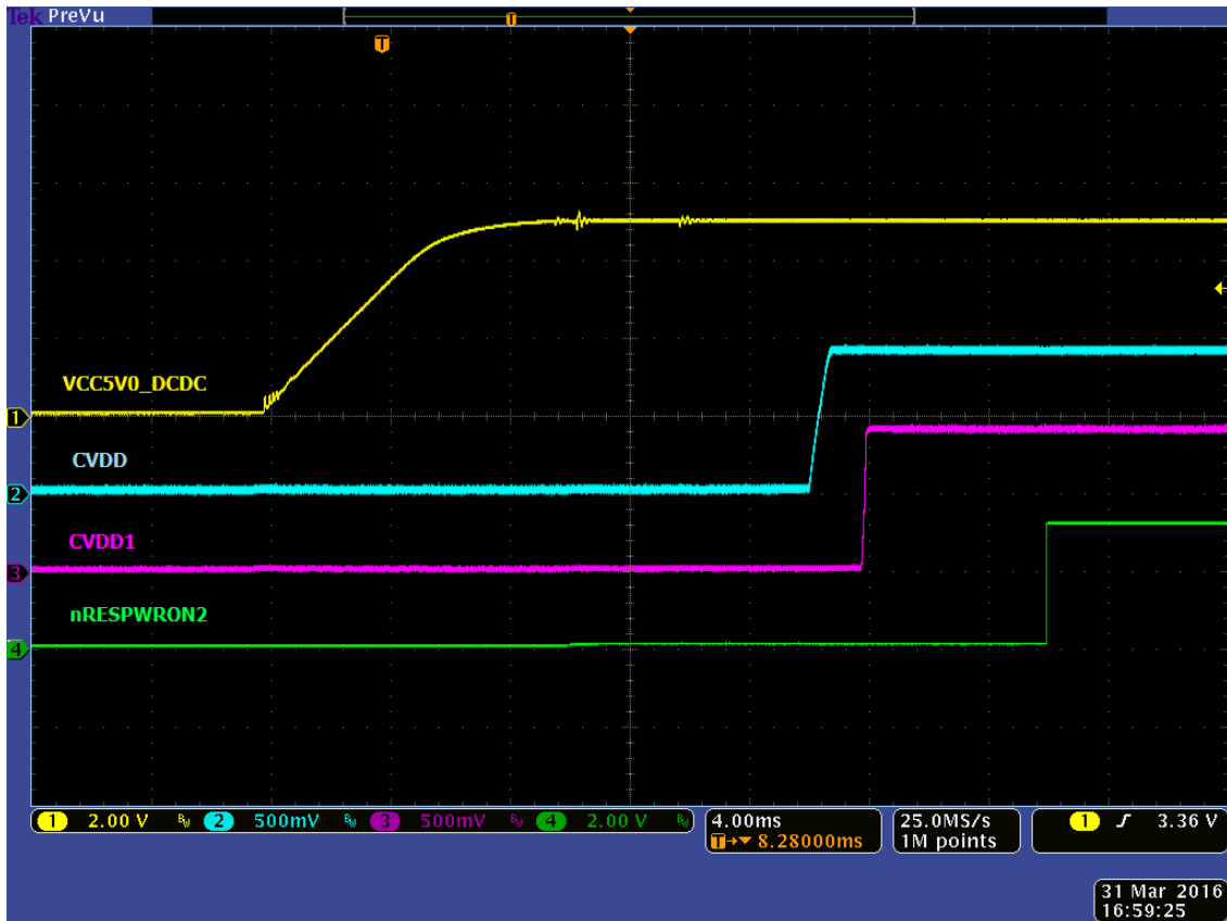
图 7. Power-On Sequence for the TPS65911x With nRESPWRON2
