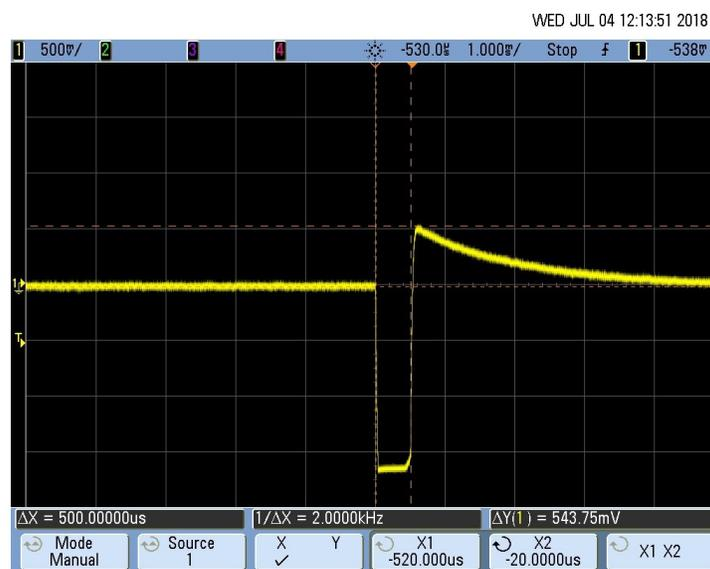
图 41. Negative Pace Signal From the Patient Simulator Interfaced With ADS1292
