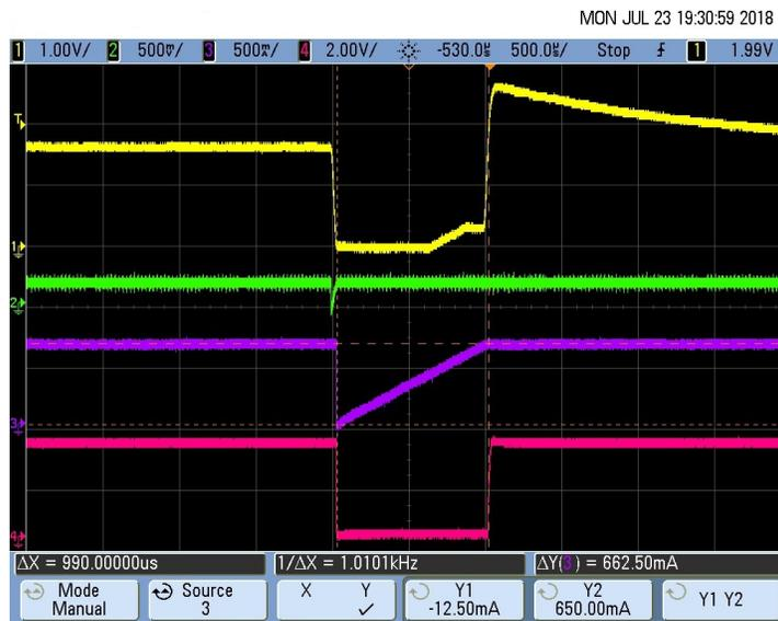
图 82. Negative Pace Signal Detection - Negative Pace Pulse Detected by setting the Polarity Check (CH-6) Output of the DAC Low
