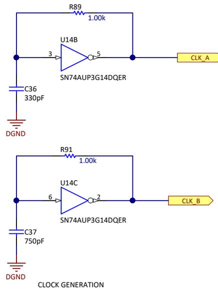
图 30. Circuitry Implemented to Generate Onboard Counter Clocks
