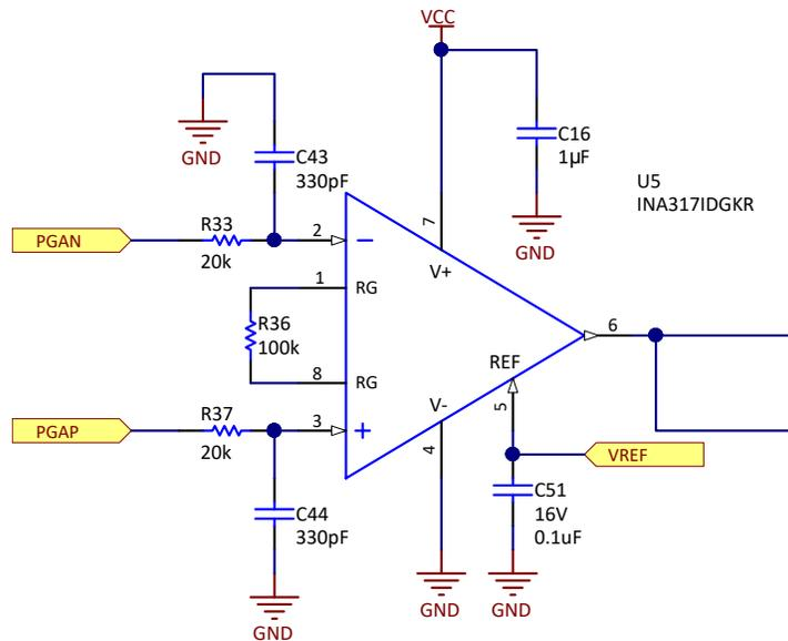
图 11. Differential to Single-Ended Conversion Circuit
