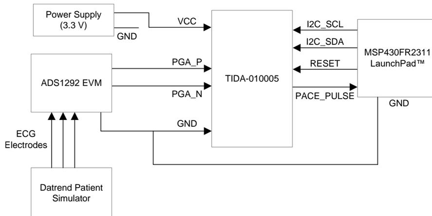
图 35. Test Setup to Evaluate the TIDA-010005 Using ADS1292 EVM and Patient Simulator
