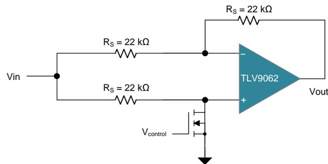
图 21. Polarity Reversal Circuit Explanation
