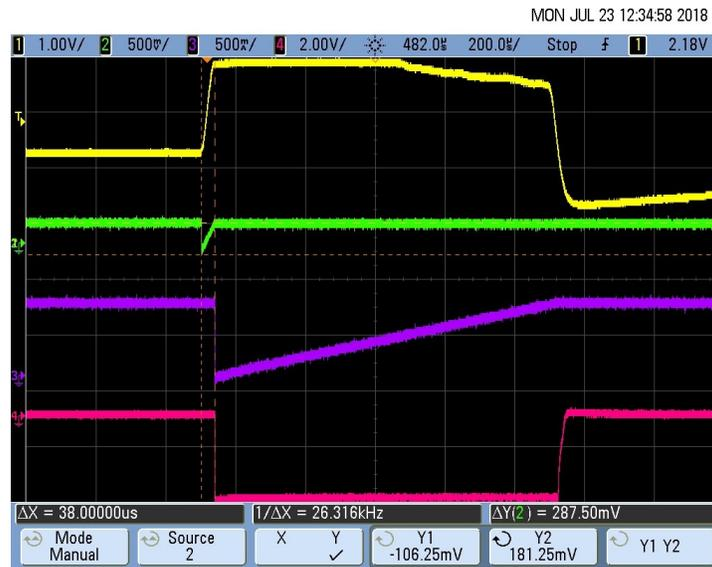
图 70. Pacemaker Detection Output (Rise Time  $T_R$ ) for 16-mV, 1-ms Pace Pulse
