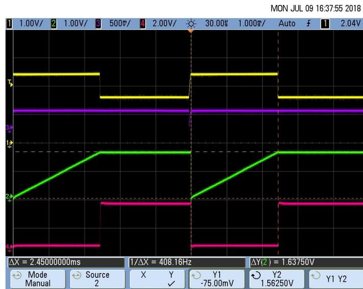
图 51. Pulse Duration Measurement of the Pace Pulse ( $T_D = 2.5$  ms)
