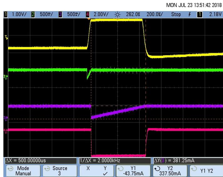
图 69. Pacemaker Detection Output (Pulse Duration  $T_D$ ) for 16-mV, 500- $\mu$ s Pace Pulse
