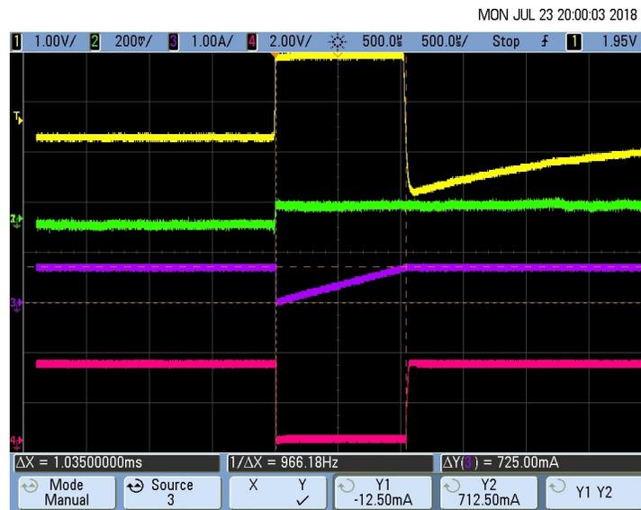
图 75. Pacemaker Detection Output (Pulse Duration  $T_D$ ) for 50-mV, 1-ms Pace Pulse
