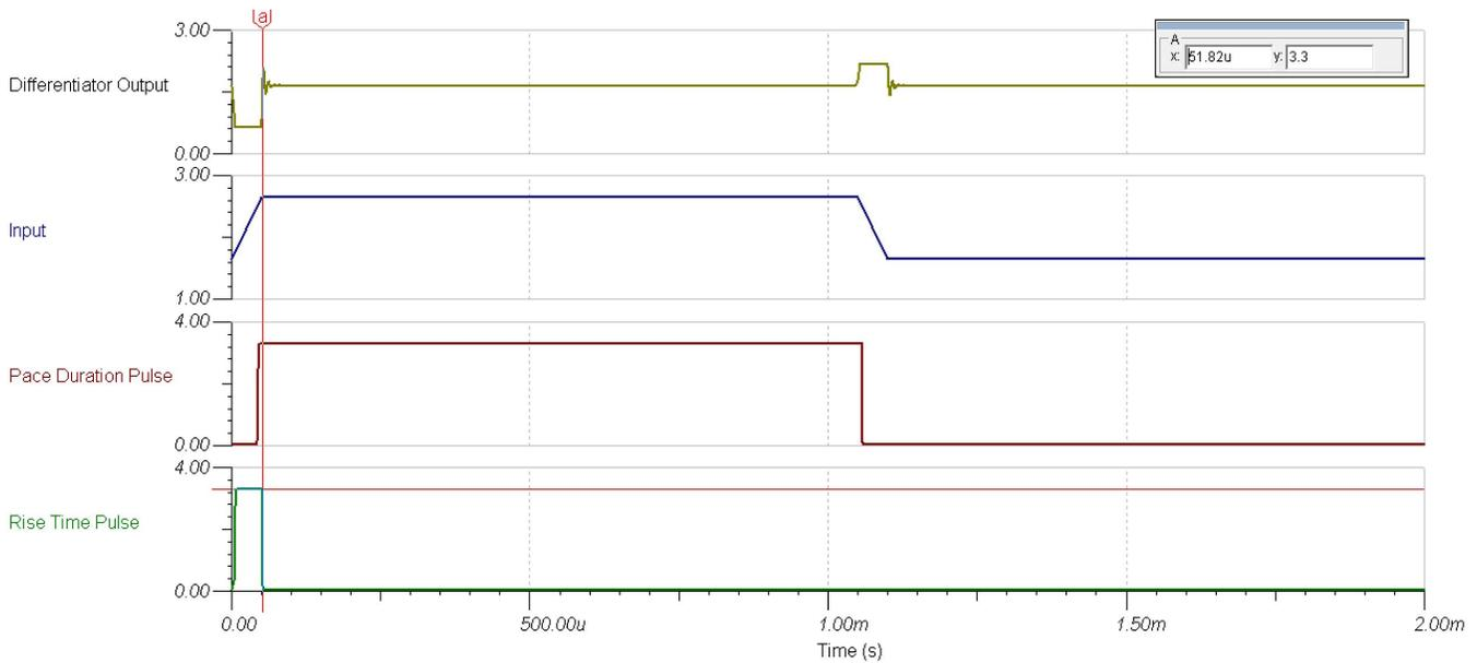
图 29. Simulation Output of the Signal Measurement Section Till TTL Pulse Generation
