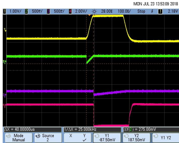
图 66. Pacemaker Detection Output (Rise Time  $T_R$ ) for 16-mV, 200- $\mu$ s Pace Pulse
