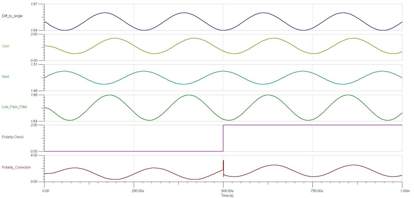
图 25. TINA-TI™ Simulation Output Characteristics of Entire Signal Processing Section
