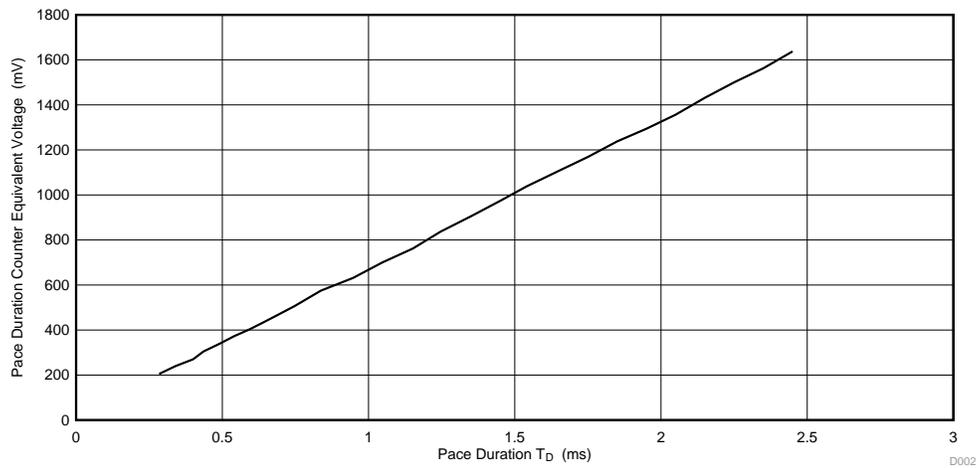
图 52. Equivalent Analog Voltage of the Pulse Duration Counter (mV) vs the Pulse Duration  $T_D$  (ms)
