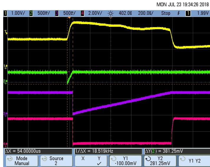
图 62. Pacemaker Detection Output (Rise Time  $T_R$ ) for 8-mV, 1-ms Pace Pulse
