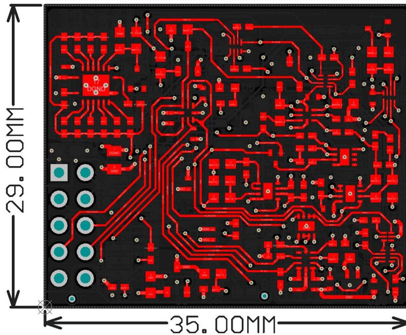
图 87. Top Layer of the Reference Board
