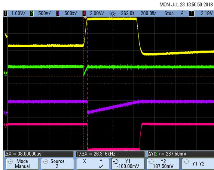
图 68. Pacemaker Detection Output (Rise Time  $T_R$ ) for 16-mV, 500- $\mu$ s Pace Pulse
