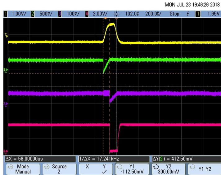
图 56. Pacemaker Detection Output (Rise Time  $T_R$ ) for 8-mV, 100-μs Pace Pulse
