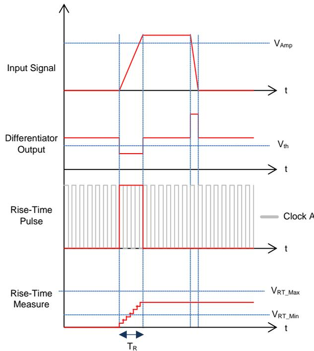
图 5. Rise Time Pulse Generation and Measurement
