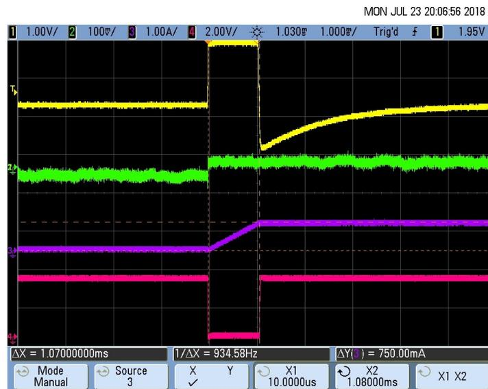
图 77. Pacemaker Detection Output (Pulse Duration  $T_D$ ) for 500-mV, 1-ms Pace Pulse
