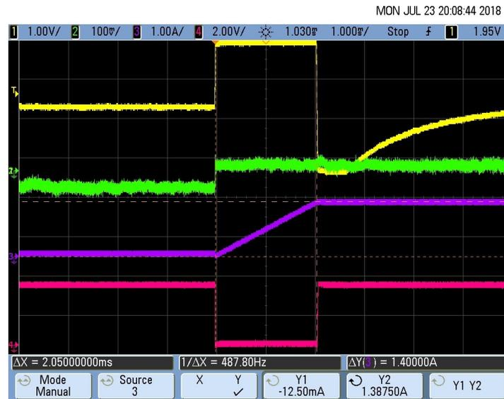
图 80. Pacemaker Detection Output (Pulse Duration  $T_D$ ) for 700-mV, 2-ms Pace Pulse
