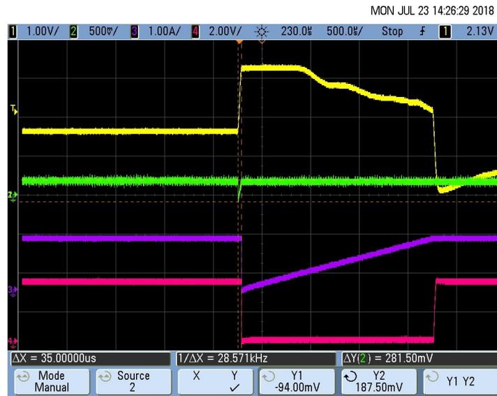
图 72. Pacemaker Detection Output (Rise Time  $T_R$ ) for 16 mV, 2 ms Pace Pulse
