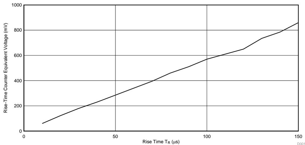
图 47. Equivalent Analog Voltage of the Rise Time Counter (mV) vs the Rise Time  $T_R$  ( $\mu s$ )
