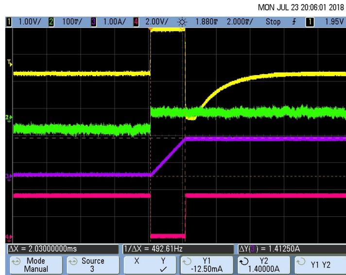
图 78. Pacemaker Detection Output (Pulse Duration  $T_D$ ) for 500-mV, 2-ms Pace Pulse
