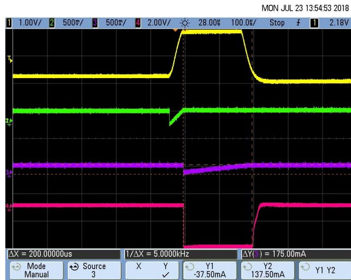
图 67. Pacemaker Detection Output (Pulse Duration  $T_D$ ) for 16-mV, 200- $\mu$ s Pace Pulse
