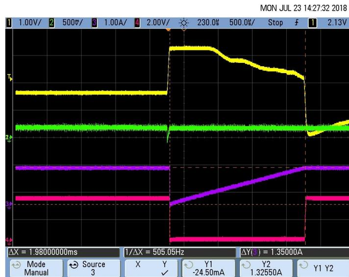
图 73. Pacemaker Detection Output (Pulse Duration  $T_D$ ) for 16 mV, 2 ms Pace Pulse
