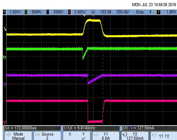
图 59. Pacemaker Detection Output (Pulse Duration  $T_D$ ) for 8-mV, 200- $\mu$ s Pace Pulse
