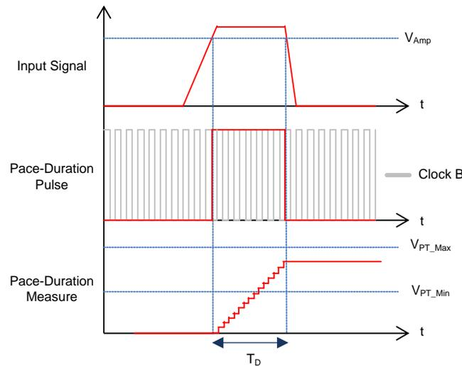
图 6. Pace Duration Pulse Generation and Measurement
