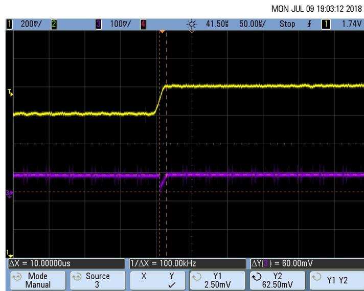
图 46. Rise Time Measurement of the Pace Signal ( $T_R = 10 \mu s$ )
