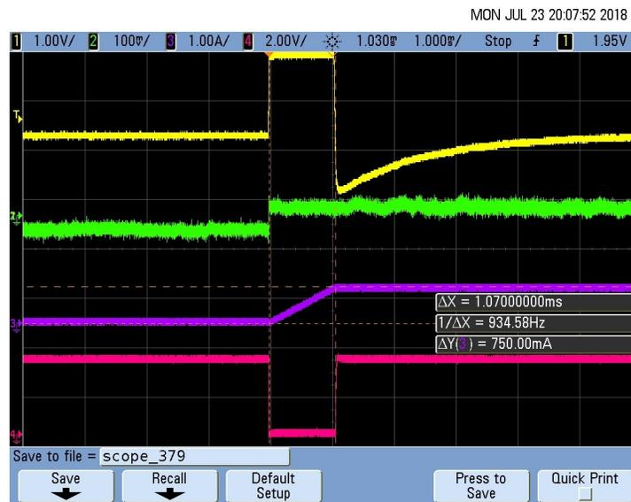
图 79. Pacemaker Detection Output (Pulse Duration  $T_D$ ) for 700-mV, 1-ms Pace Pulse
