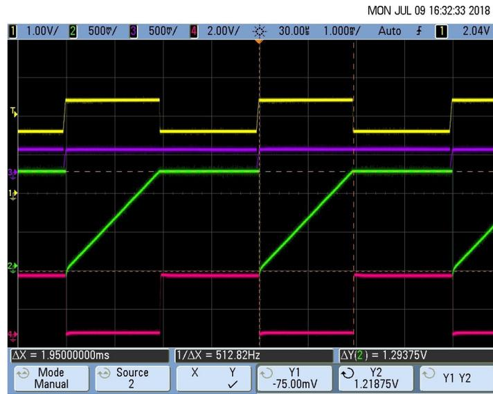
图 50. Pulse Duration Measurement of the Pace Pulse ( $T_D = 2$  ms)
