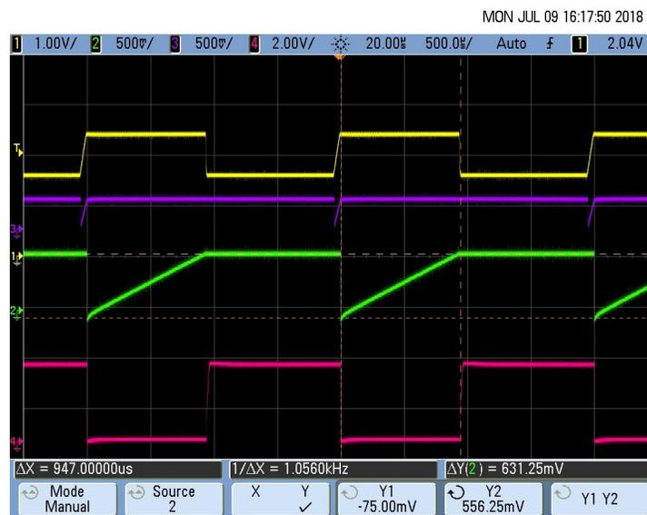
图 49. Pulse Duration Measurement of the Pace Pulse ( $T_D = 1 \text{ ms}$ )
