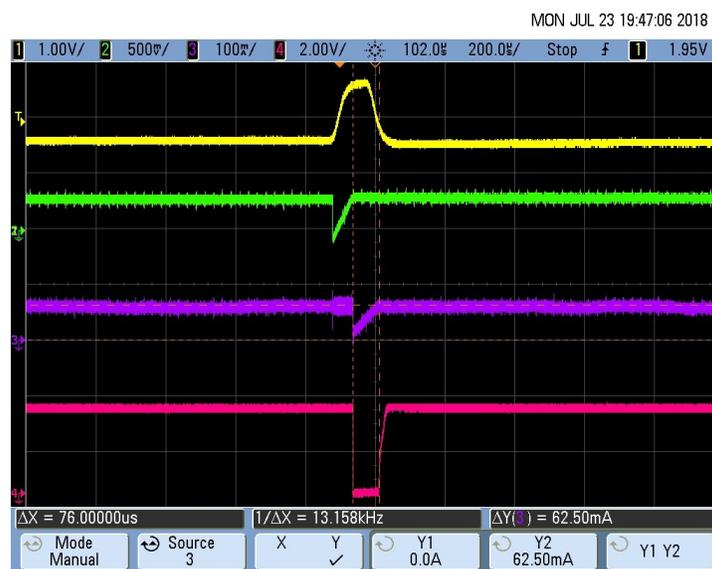
图 57. Pacemaker Detection Output (Pulse Duration  $T_D$ ) for 8-mV, 100-μs Pace Pulse
