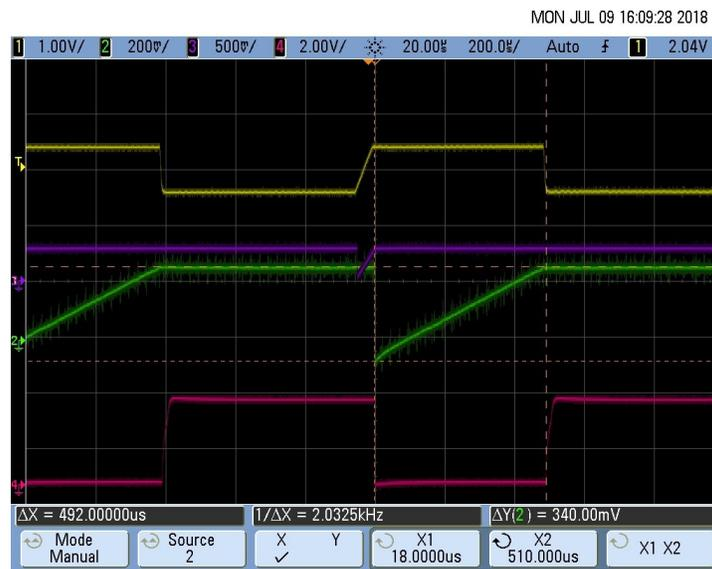
图 48. Pulse Duration Measurement of the Pace Pulse ( $T_D = 0.5 \text{ ms}$ )
