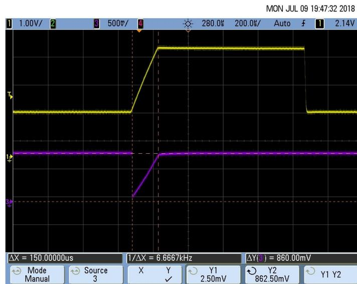
图 42. Rise Time Measurement of the Pace Signal ( $T_R = 150 \mu s$ )
