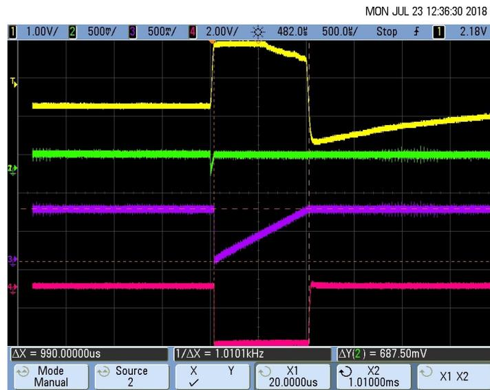
图 71. Pacemaker Detection Output (Pulse Duration  $T_D$ ) for 16-mV, 1-ms Pace Pulse
