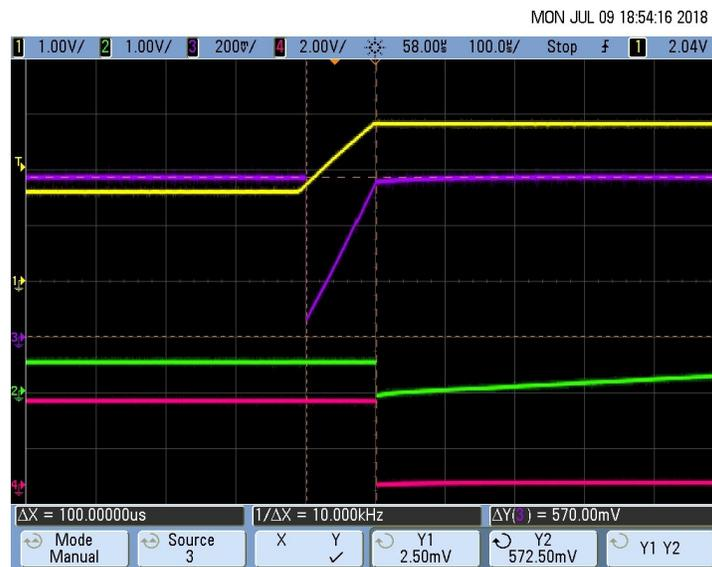
图 43. Rise Time Measurement of the Pace Signal ( $T_R = 100 \mu s$ )
