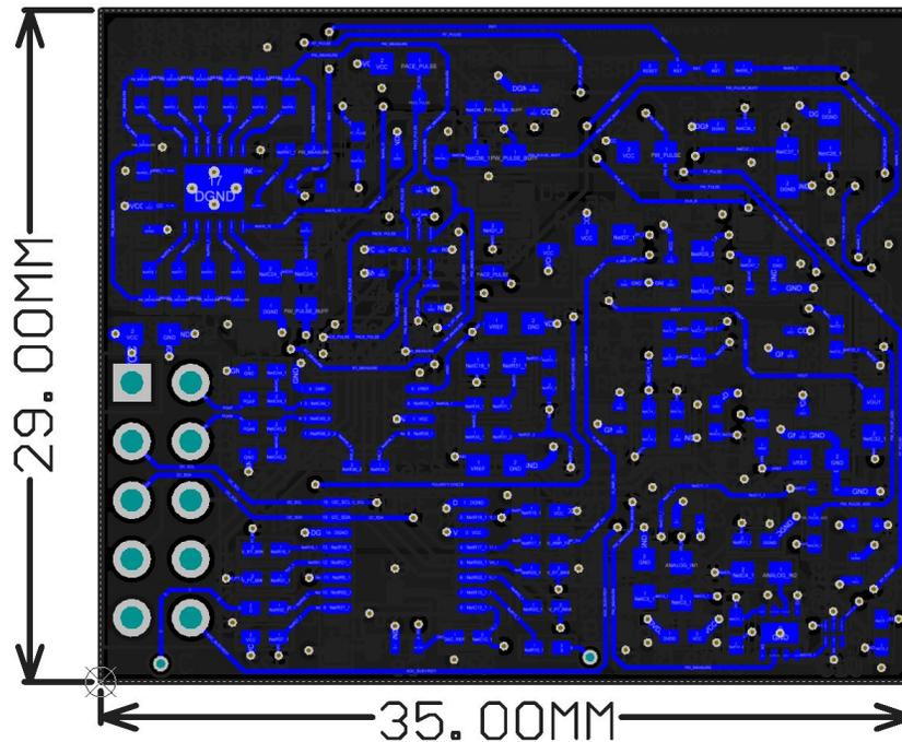
图 88. Bottom Layer of the Reference Board
