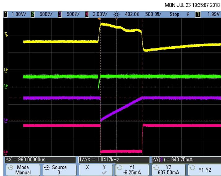
图 63. Pacemaker Detection Output (Pulse Duration  $T_P$ ) for 8-mV, 1-ms Pace Pulse
