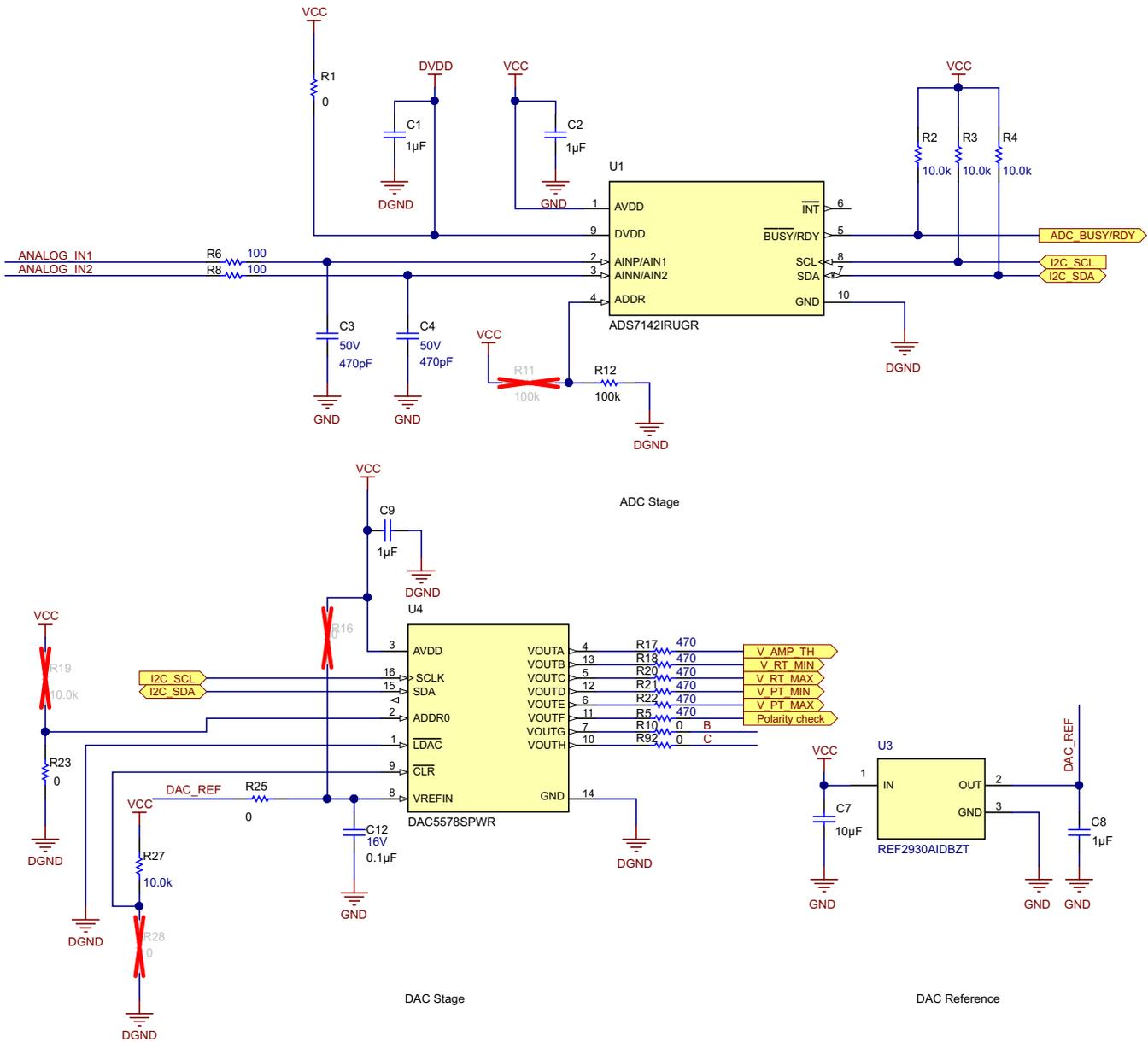
图 31. ADC & DAC Implementation in the Reference Design
