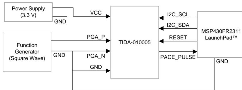
图 34. Test Setup to Evaluate the TIDA-010005 Using Function Generator
