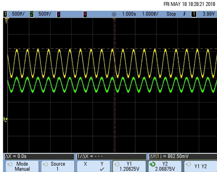
图 36. Output Characteristics of Differential to Single-Ended Converter (INA317)
