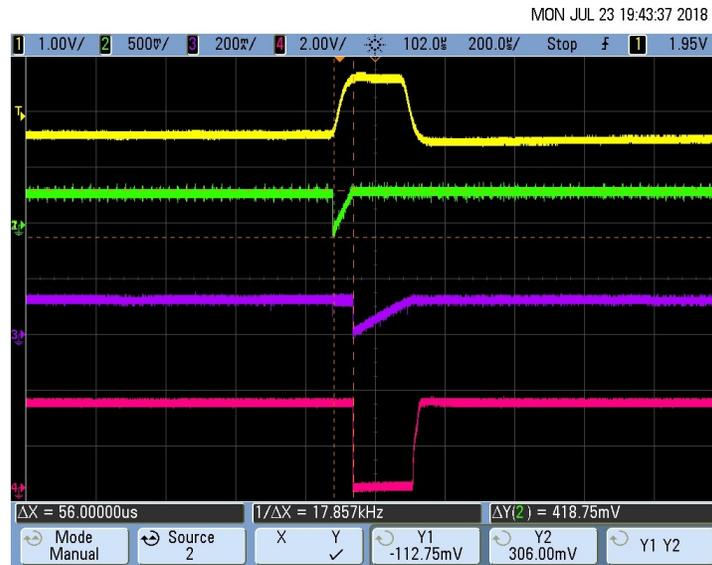
图 58. Pacemaker Detection Output (Rise Time  $T_R$ ) for 8-mV, 200- $\mu$ s Pace Pulse
