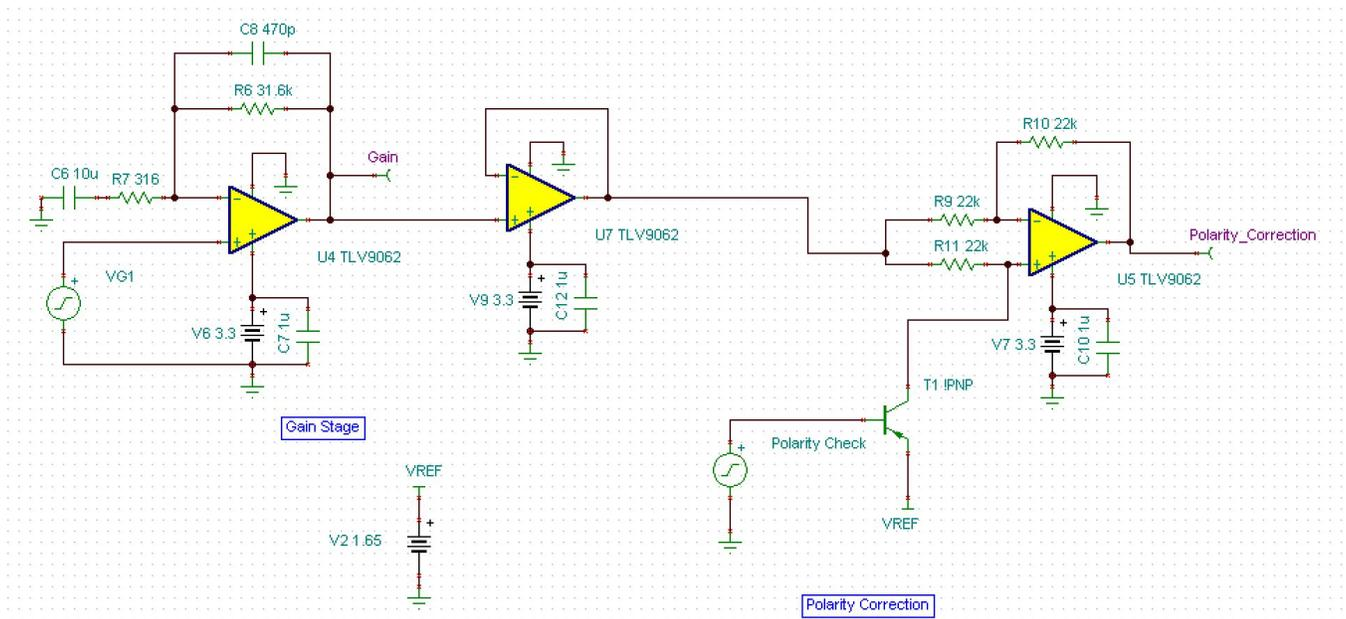
图 22. TINA-TI™ Simulation Schematic Gain and Polarity Correction Circuit
