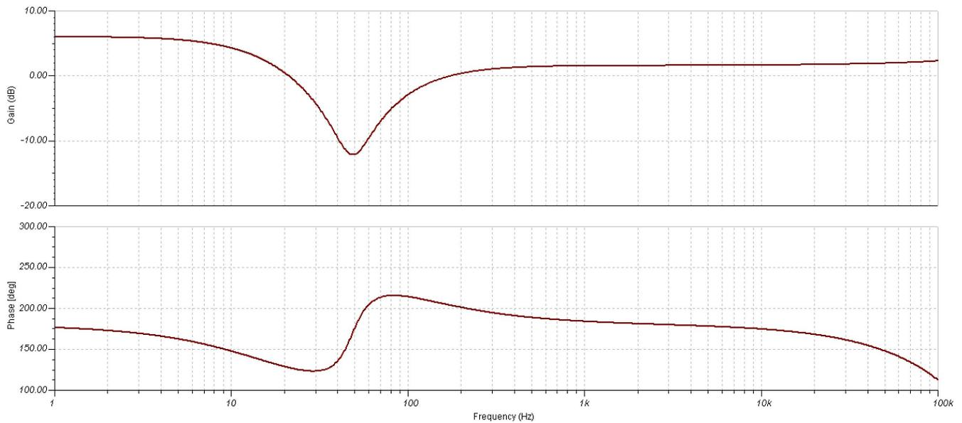
**图 19. Frequency and Phase Response of the 50-Hz Notch Filter From 1 Hz to 100 kHz**
