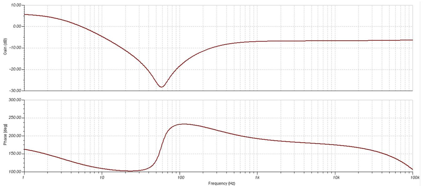
图 17. Frequency and Phase Response of the 60-Hz Notch Filter From 1 Hz to 100 kHz
