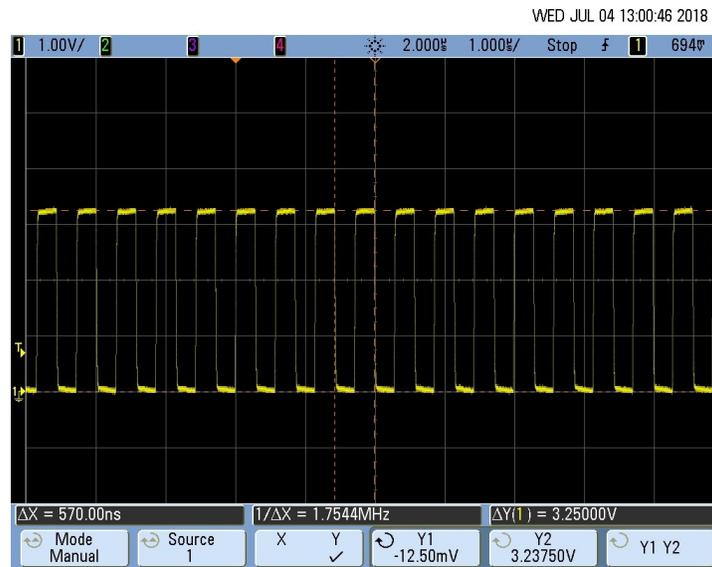
图 53. Clock (CLK A) Input to Rise Time Counter
