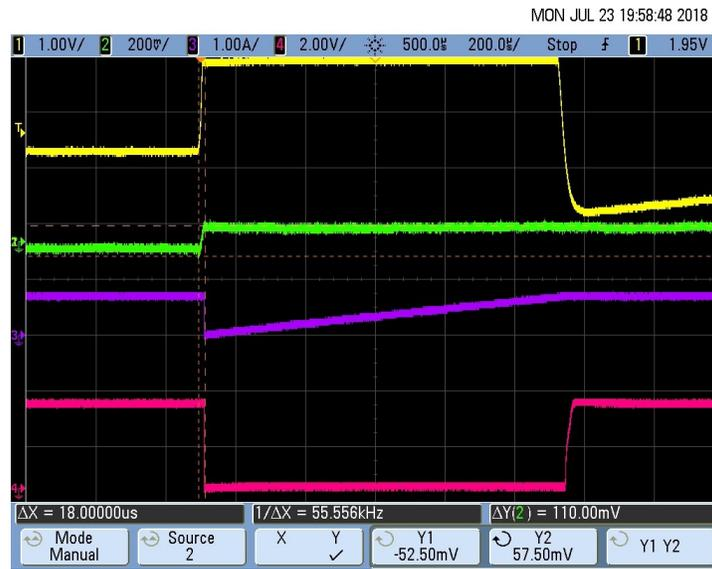
图 74. Pacemaker Detection Output (Rise Time  $T_R$ ) for 50-mV, 1-ms Pace Pulse
