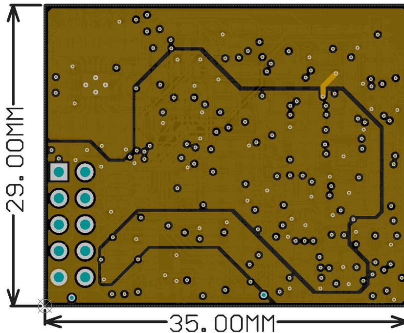
图 85. Ground Planes of the Reference Design Board
