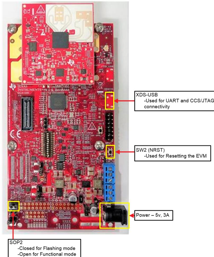
**图 8. TIDUEP0103 Gesture HMI Hardware Setup**
