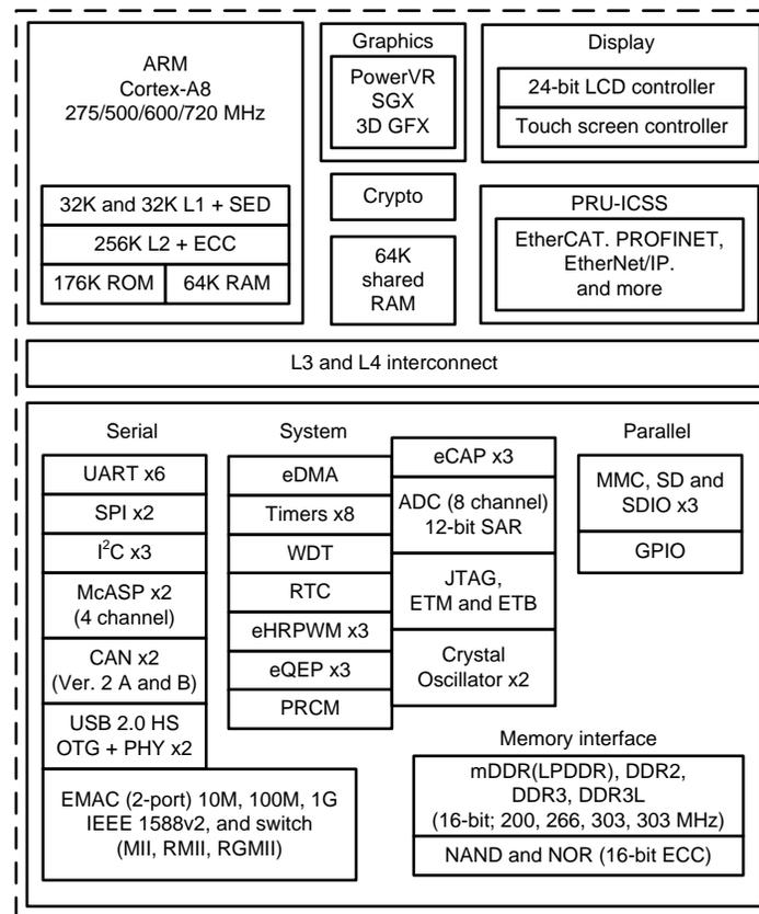
The microprocessor unit (MPU) subsystem is based on the Arm® Cortex®-A8 processor and the PowerVR SGX™ Graphics Accelerator subsystem provides 3D graphics acceleration to support display and gaming effects.
