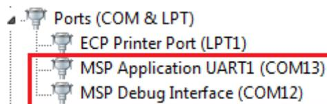
Figure 7. Application Backchannel UART in Device Manager
