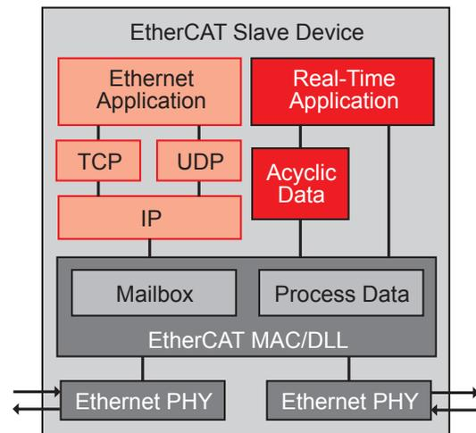
**Figure 3.** Components of an EtherCAT node.
