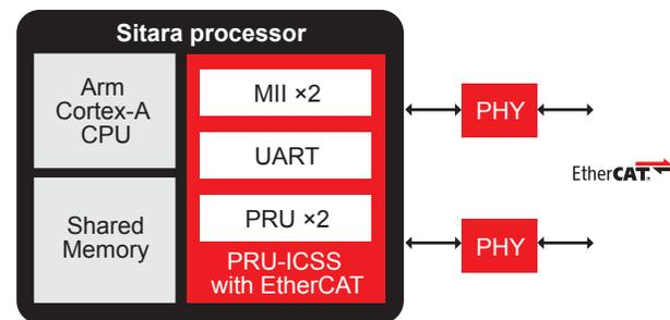
**Figure 7.** EtherCAT slave on TI Sitara processors.
