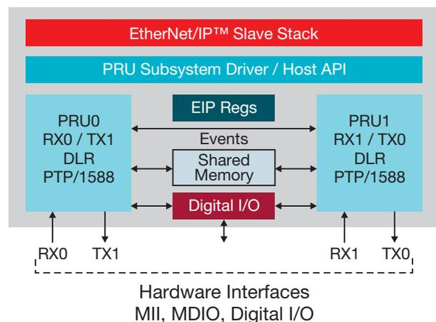
**Figure 10.** Firmware architecture.
