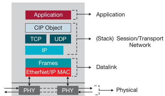
**Figure 5.** EtherNet/IP node.
