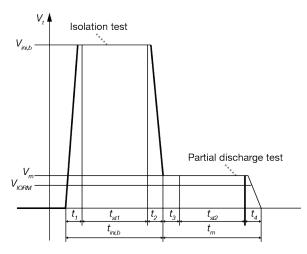
Figure 3. Method-B1 routine production test performed on all parts.
