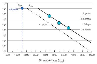
Figure 5. Time Dependent Dielectric Breakdown (TDDB). Circles are the time for 63% of units to break down. The dashed line represents 1ppm projections from the Weibull analyses.
