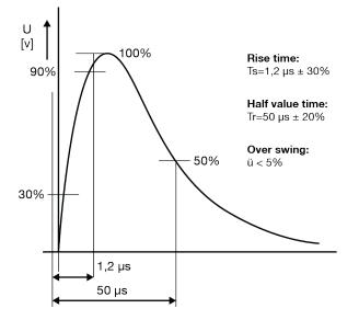
Figure 6. Surge test waveform.
