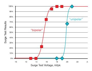
*Figure 7.* Surge breakpoint statistical assessment, by both "unipolar" and "bipolar" surge test methods .
