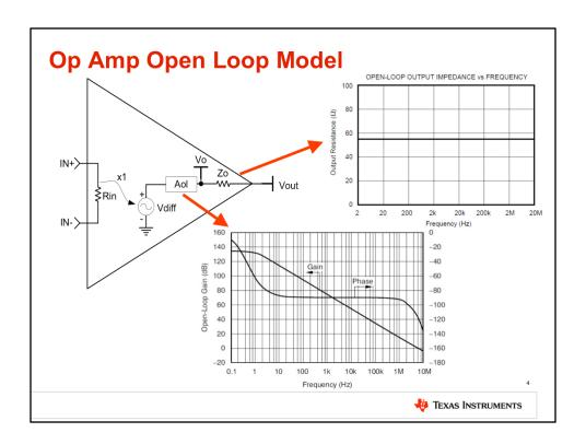
It is helpful to use an intuitive model for the op amp when performing ac stability analysis because of the complexity of modern op amps. In this simplified "stability" model, the differential input voltage applied to the inputs is passed to the amplifier output stage where it passes through the amplifier open-loop gain, followed by the open-loop output impedance before it reaches the output terminal.
