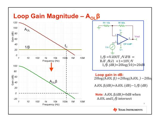
First we can consider the loop gain magnitude using a Bode plot. Using the same circuit as before, we have a gain of 10V/V, or 20dB, so 1/B is a constant 20dB over frequency. The circuit's Aol is also shown. To find the magnitude of AolB, we can simply subtract 1/B from Aol. This might not seem intuitive, but the mathematical relationship shown on the right side of the slide proves this using the properties of logarithms.
