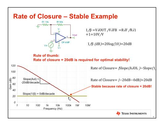
We can also analyze the standard non-inverting amplifier circuit from earlier in the lecture using the rate of closure method.
