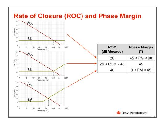
As shown in the previous slides, rate of closure and phase margin are directly related to each other allowing us to predict one value based on the other. This slide gives three different examples of rate of closure and their corresponding phase margins.
