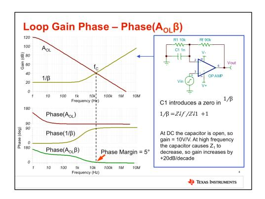
To measure the phase margin, we need to know the loop gain phase, or phase of  $Aol\beta$ , over frequency. Using the same log properties as before, we can simply subtract the phase of 1/B from the phase of Aol to get the phase of AolB.
