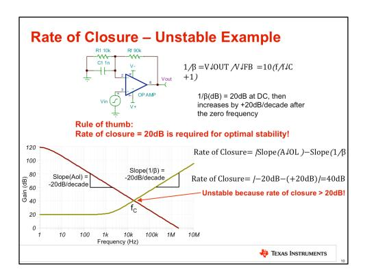
This method is called rate of closure analysis. To use this method, we only need to consider the magnitude plots of AoI and 1/B. These plots have well-defined slopes due to the poles and zeros in their transfer functions. By analyzing the rate of closure of AoI and 1/B at fC, the point where they intersect, we can quickly determine the stability of a circuit. The rule of thumb for this method is that the rate of closure at fc must equal 20dB for optimal stability.
