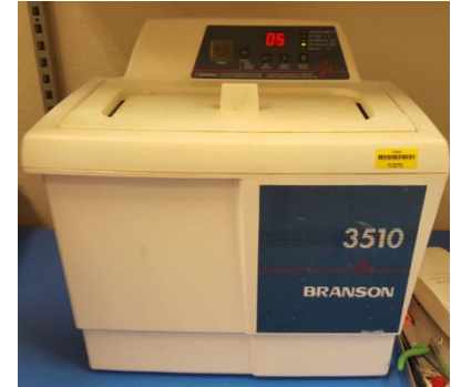
Figure 12-2 An example sonic bath tool, Branson 3510
