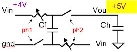
Regulate Gate Drive on 2 Switches to Control Vout
