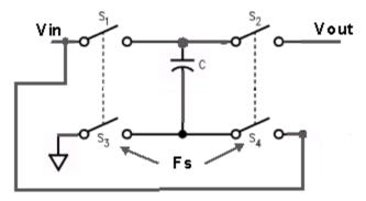
By swapping V<sub>in</sub> and V<sub>out</sub>, the same doubler circuit will give half gain
