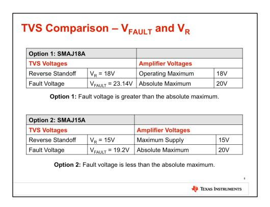
We now must compare the TVS voltages to the op-amp specifications. Recall that the TVS reverse standoff of 18V was selected to match the op amp operating supply voltage of 18V. We determined that the fault voltage is actually 23.14V using linear interpolation between known points on its I-V curve. For best protection, the fault voltage should be less than the op amp absolute maximum voltage, unfortunately, this TVS fault voltage is above the op amp absolute maximum of 20V.
