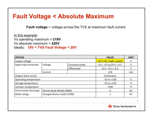
Let's take a look at the absolute maximum specifications for the OPA192. Recall from the last slide that the OPA192's operating voltage is  $\pm 18V$ . The absolute maximum for this device is  $\pm 20V$ . So, if the amplifier supply is normally at  $\pm 18V$ , then the TVS diode must be fully off at 18V. However, the TVS needs to turn on to protect the amplifier before the supply reaches the absolute maximum of  $\pm 20V$ .
