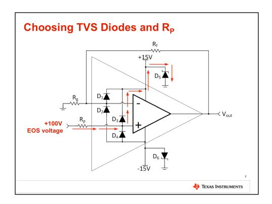
The objective in selecting the TVS diode is to make sure that the diode is off and has minimal leakage during normal operation, but turns on and limits the supply voltage under overstress conditions. The objective in selecting the resistor is to limit the input current to less than 10mA.
