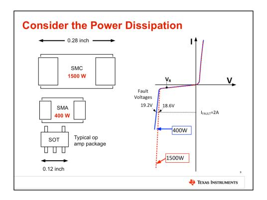
Ideally the TVS reverse standoff voltage and fault voltage would be very close to each other, since op amps often have operating conditions which are near the absolute maximum voltage. However, this isn't always the case. Thankfully we can consider TVS diodes with different power ratings. Increasing the power rating increases the slope of the curve in the reverse breakdown region, which will move the fault voltage closer to the reverse standoff voltage.
