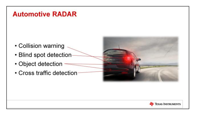
In the continually-progressing world of automotive safety, RADAR technology is often used to detect all kinds of conditions while driving. RADAR can be used for (CLICK) checking for an impending collision, (CLICK) monitoring cars that might be in a blind spot, (CLICK) detecting objects that can't be seen over the hood or behind the trunk, (CLICK) or watching cross traffic to avoid an accident while reversing out of a parking space, to name a few. So, how does RADAR accomplish these tasks?
