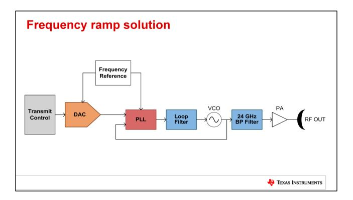
A precision DAC is needed to finely tune the oscillation circuit that generates the RADAR signal. The DAC reference input is coupled to the reference frequency of the PLL and voltage controlled oscillator. Therefore, as the DAC changes its code from 0 to full scale, each code transition makes a small change to the output frequency of the VCO, generating the required frequency ramp. The VCO output is then applied to a 77 GHz band pass filter, and then amplified out through the transmitter.
