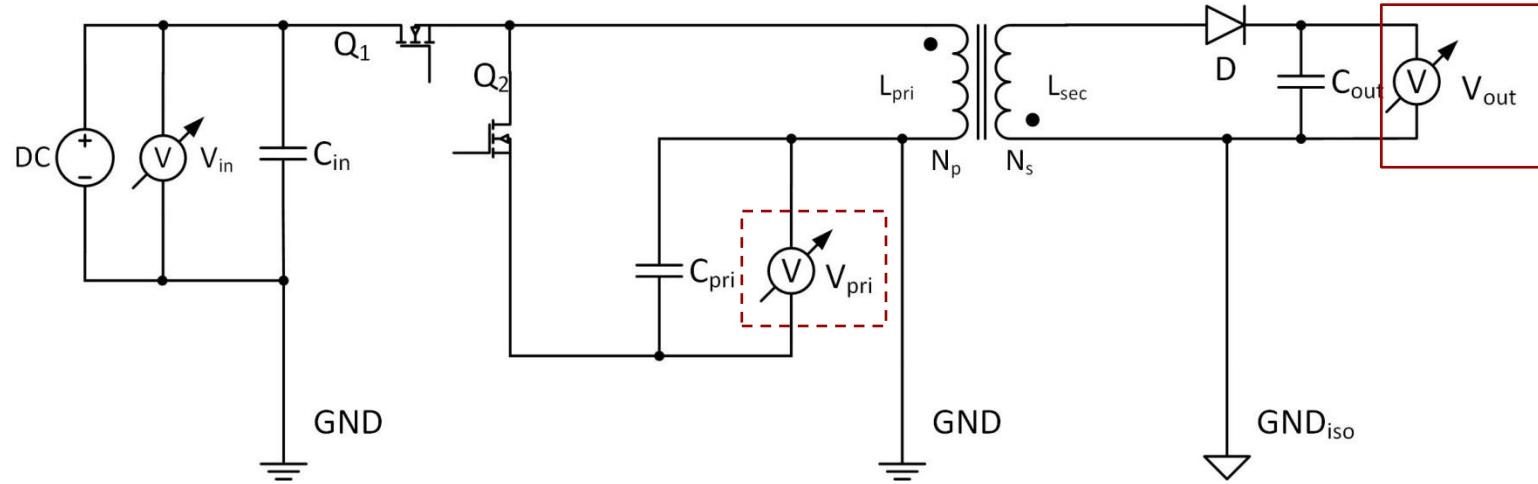
$$-V_{pri} = V_{in} \cdot \frac{t_{on}}{t_{off}} = V_{in} \cdot \frac{D}{1 - D}$$
