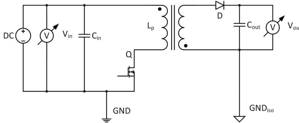
$$\frac{V_{out}}{V_{in}} = D \cdot \sqrt{\frac{T \cdot V_{out}}{2 \cdot I_{out} \cdot L_p}}$$
