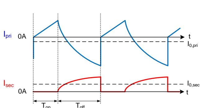
$$D = \frac{t_{\text{on}}}{t_{\text{on}} + t_{\text{off}}}$$
