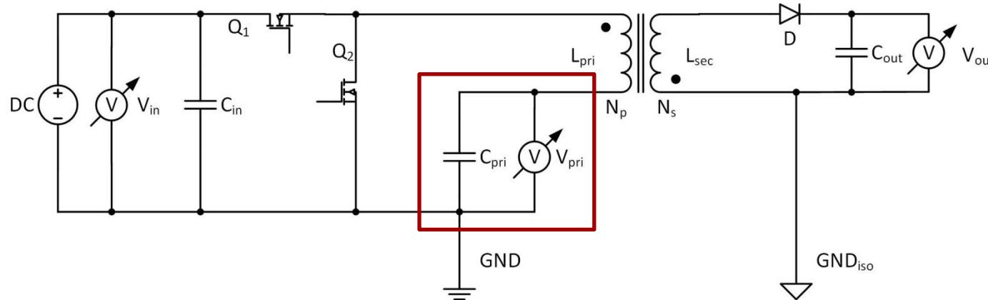
$$V_{out} = V_{pri} \cdot \frac{N_s}{N_p} - V_D$$
