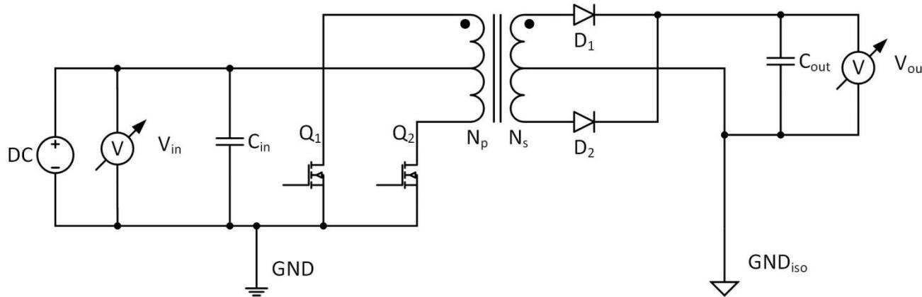
$$V_{out} = V_{in} \cdot \frac{N_s}{N_p}$$
