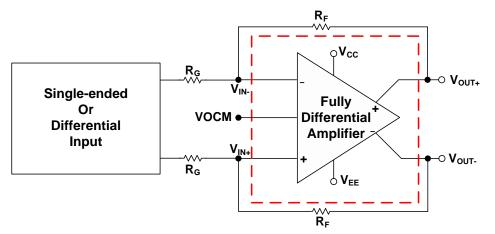
3. An FDA is operating on 5V supplies and its outputs have the ability to swing rail-to-rail. What is the maximum differential output voltage of the FDA (assume a sinusoidal signal and VOCM at mid-supply)?
