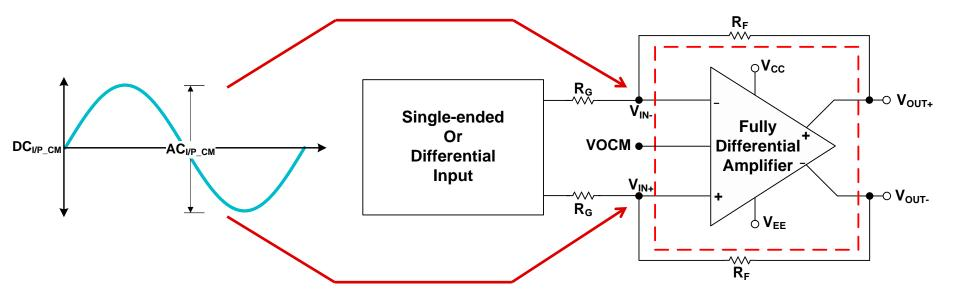
1 The voltage (DC and AC) at the inputs track each other exactly, similar to an opamp's virtual short across its inputs.
