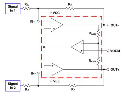
Integrated solution can offer lower noise for same power consumption and better matching for reduced balance error.
