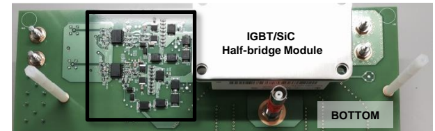
Isolated Half-bridge Drive Stage using ISO5852S-Q1 + 15A Buffer Driver
