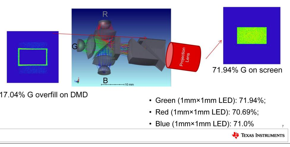
This page shows the evaluation result of the design using 1 millimeter by 1 millimeter LED. Geometric efficiency is a key performance metric that characterizes the percentage of the total rays passing through the optical system. It does not take into consideration of diffraction loss, surface reflection loss, material absorption loss, et cetera. However, with the geometric efficiency, customer can use their transmissive data together with the DMD efficiency to estimate the engine efficiency.
