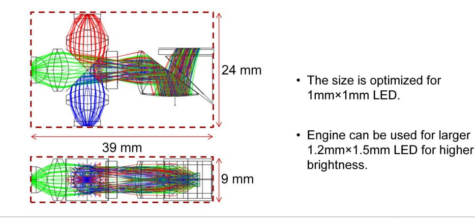
The two views on this page show the optical size of the illumination, 39 millimeter by 24 millimeter, with 9 millimeter height. To estimate the final engine size, well we need to add the other necessary mechanical and electrical components. Again, the size is optimized to achieve high efficiency for 1 millimeter by 1 millimeter LED. You can be directed to use the for 1.2 millimeter by 1.5 millimeter LED with compromised performance.
