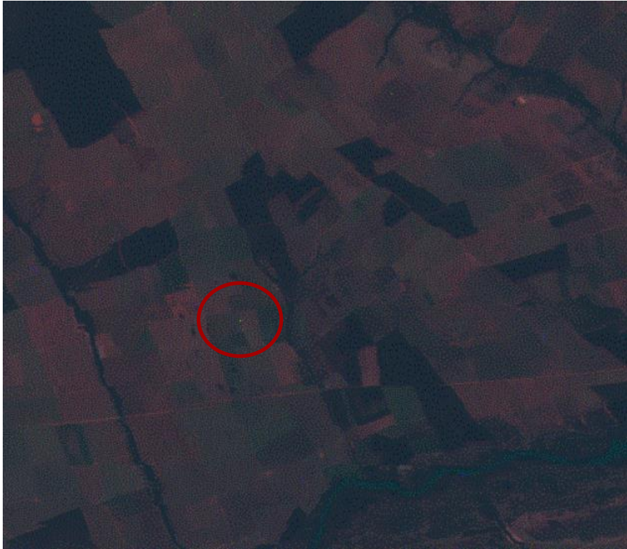
Green spot is from an SEU on the Level-0 Landsat 7 Enhanced Thematic Mapper Plus (ETM+) https://landsat.usgs.gov/single-event-upset-seu
