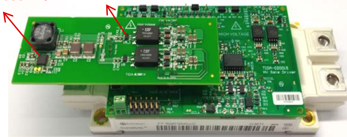
Implementation of Bias Supply Solution 3 (Buck + Push-pull)
