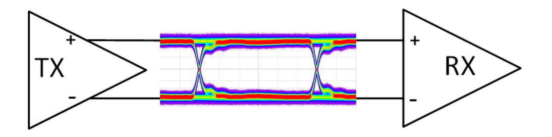
Data-dependent electrical measurement used to evaluate high-speed data quality and high-speed transmitter/receiver performance.
