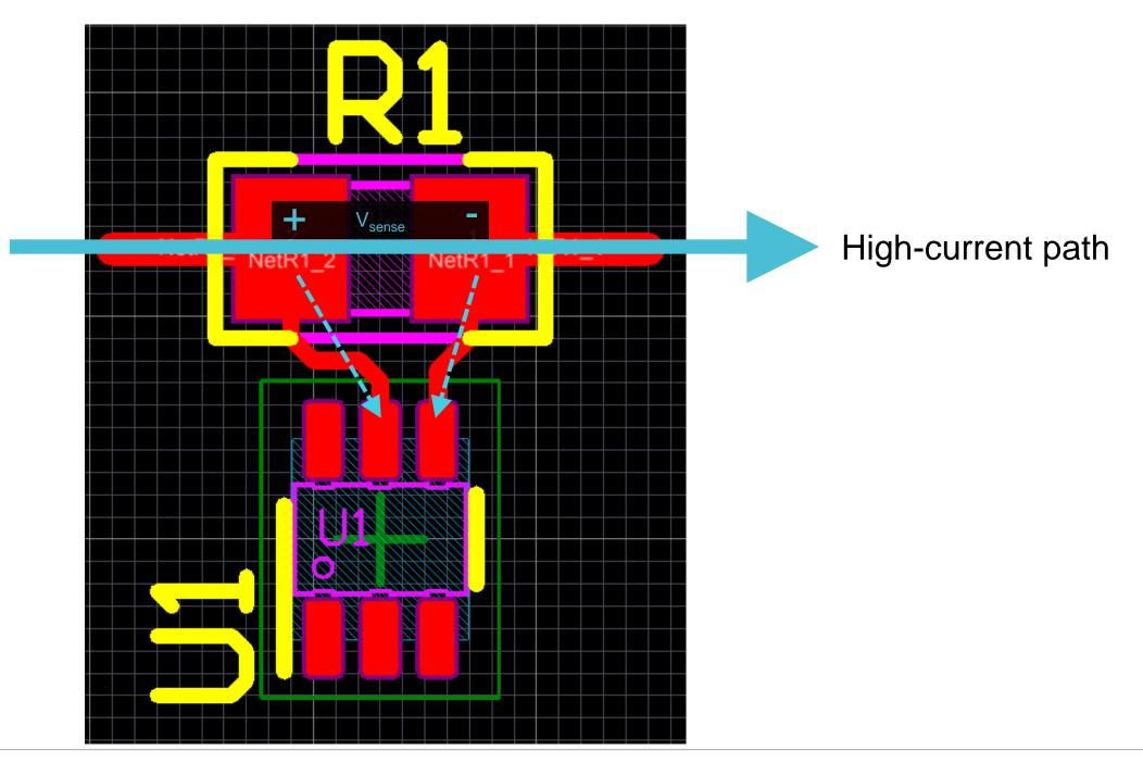
Here is an example of a good layout. Note that the shunt resistor is close to the amplifier.
