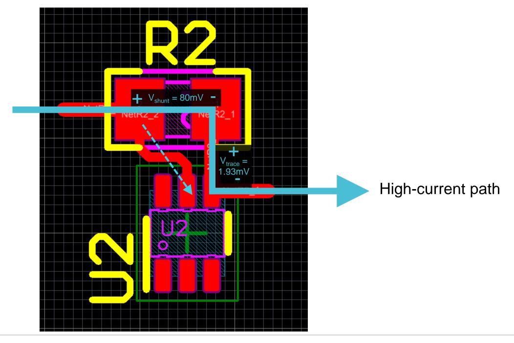
Here is an example of a bad layout. Note that the shunt resistor is still close to the amplifier.
