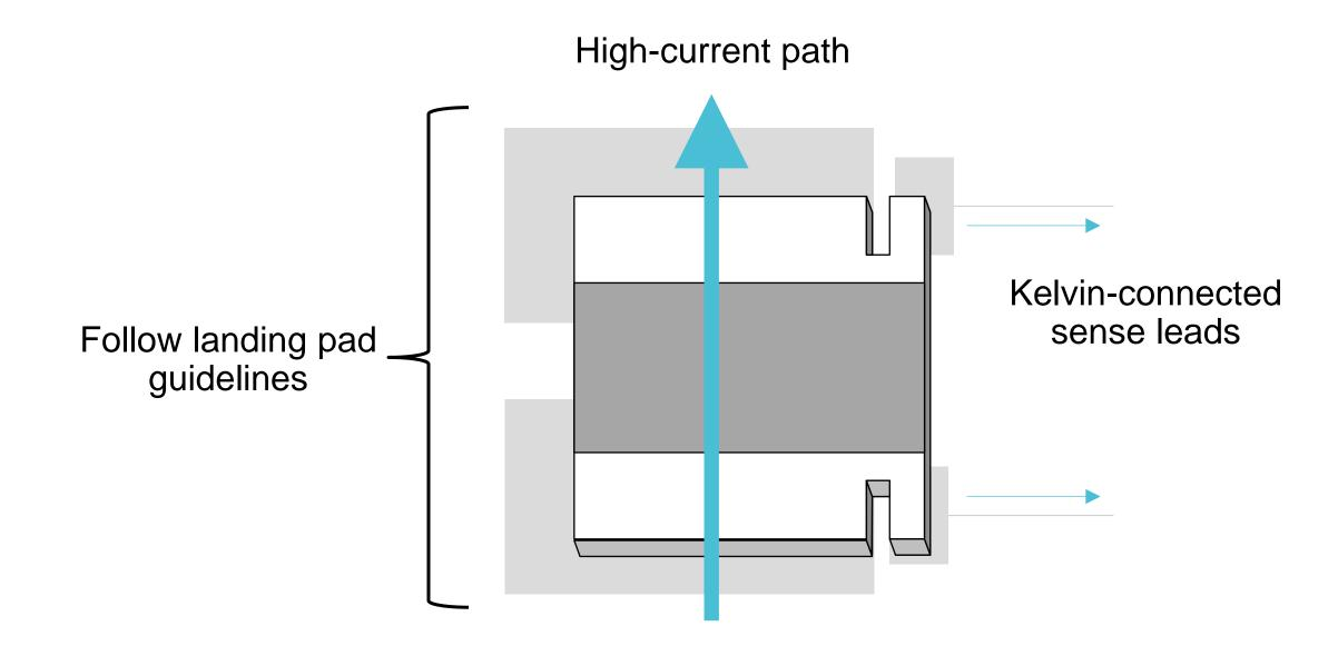
Specialty resistors often have manufacturer recommendations. In this case, the recommendations may be that there are large pads for the high current path and small pads for the Kelvin connected sense traces.
