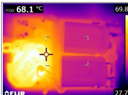
Figure 42. V_{IN} = 265 V_{AC} , Top Side (Transformer: 69 °C)
