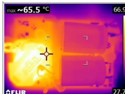
Figure 40. V_{IN} = 230 V_{AC} , Top Side (Transformer: 66 °C)
