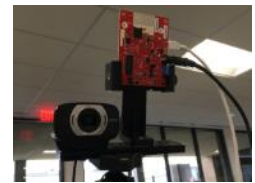
Mounting assumes 1.5-2.5m elevation, with 10 degree downtilt
