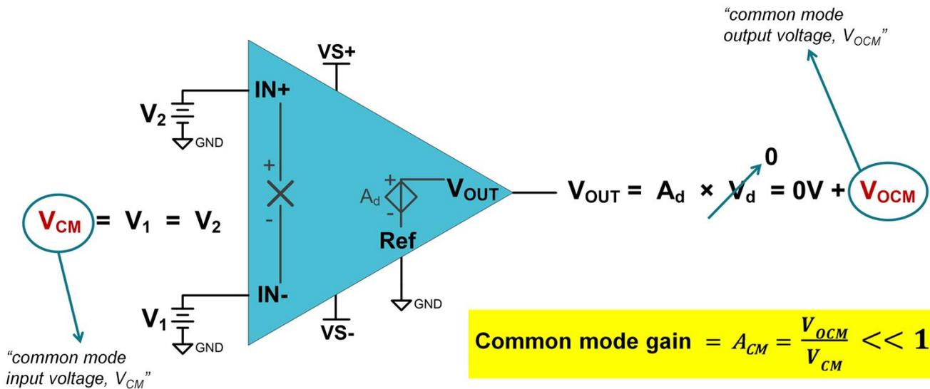
But in actuality, there will be some small voltage at the output. This is called the common mode output voltage, or  $V_{OCM}$ .
