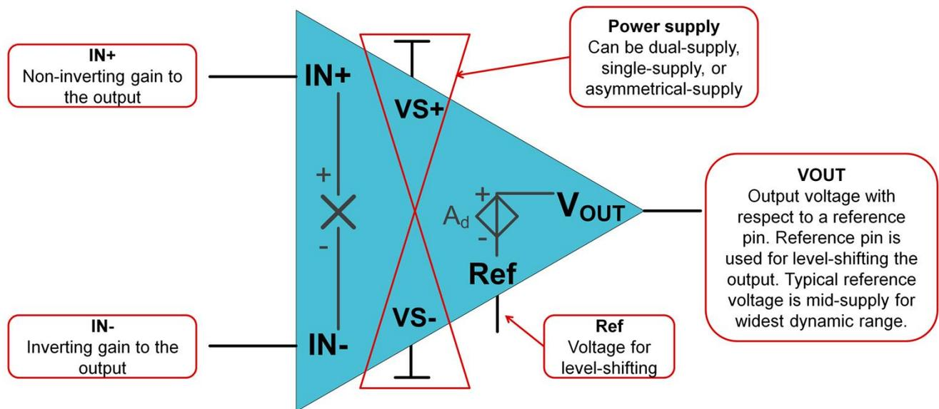
Before delving into this function, though, let us first define the various pins on an IA.
