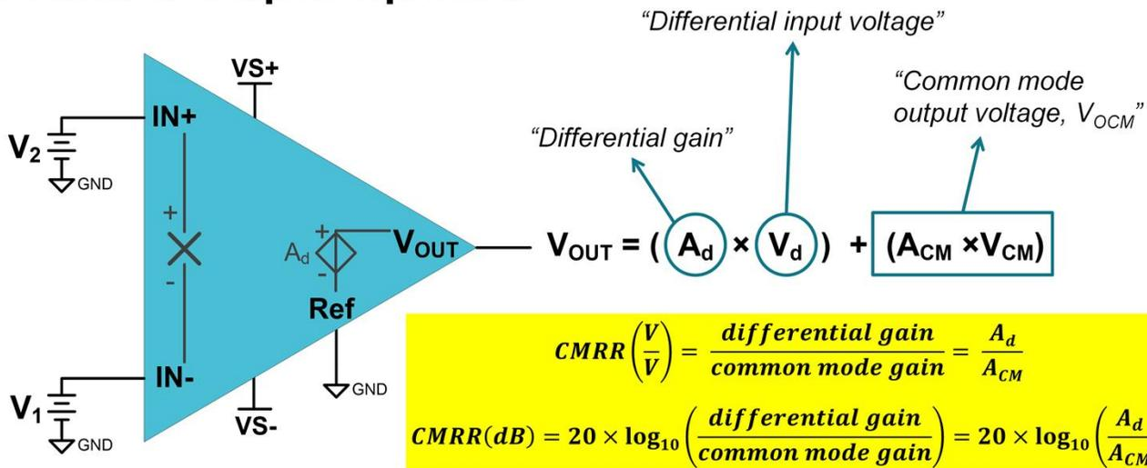
However, because of the common mode input signal dependence discussed previously, a non-ideal IA will exhibit some degree of output voltage error. This error, the “common mode output voltage”, is equal to the common mode gain multiplied by the common mode input signal.
