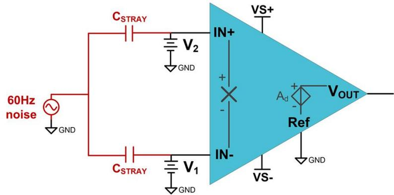
When the IA inputs are tied together to a common mode voltage, the experienced output voltage ( $V_{OCM}$ ) could be due to common mode noise sources.
