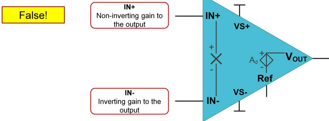
This is false. IN- means it has inverting gain to the output. IN+ has non-inverting gain to the output. Either pin can be positive or negative voltages and be greater or less than each other.
