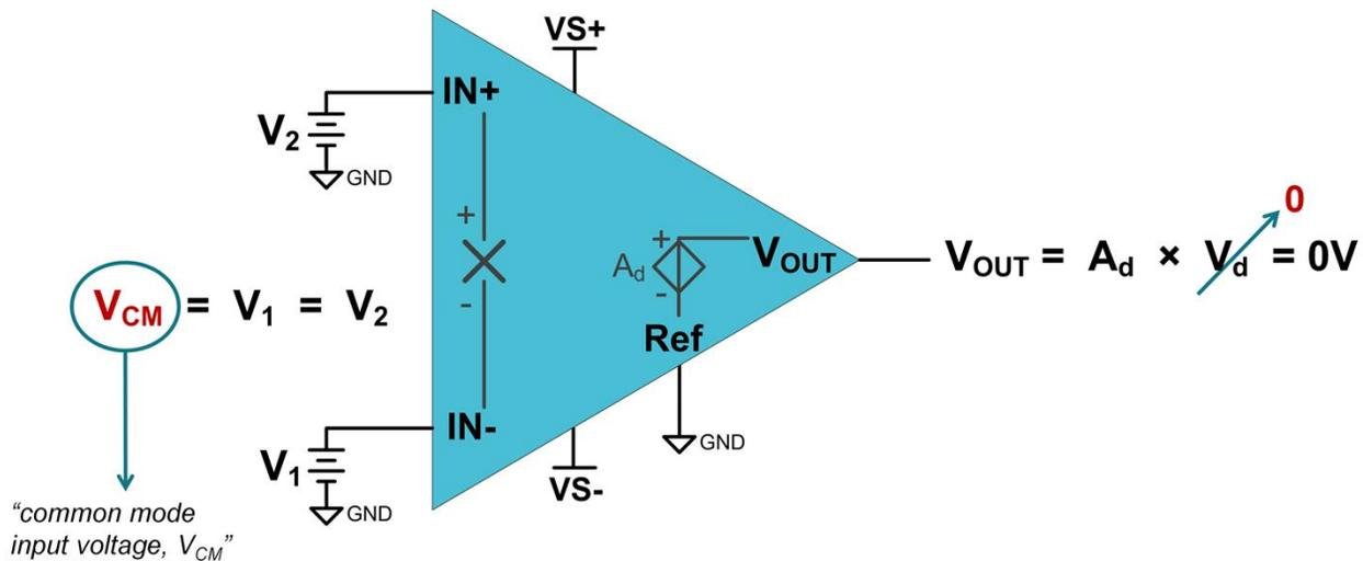
Let us examine now a case where the inputs are equal to each other, and both are tied to a common mode input voltage or  $V_{CM}$ .
