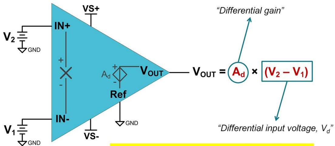
**Differential input voltage:  $V_d = V_2 - V_1$**
