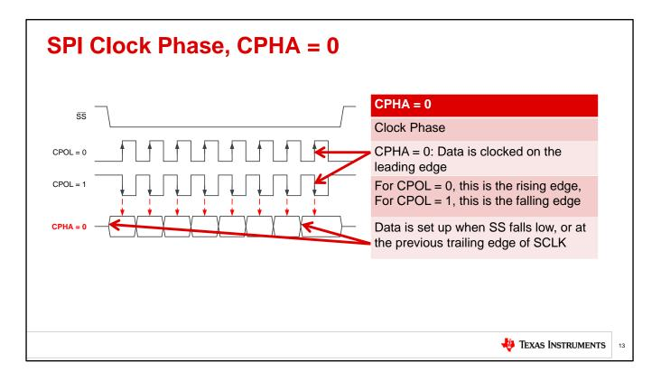
The second parameter, CPHA, determines the clock phase for which the data is acquired. For the CPHA equal to zero, data is captured on the leading edge of the clock pulse. Data is set up on the trailing edge of SCLK for the first bit, when SS bar is set low.
