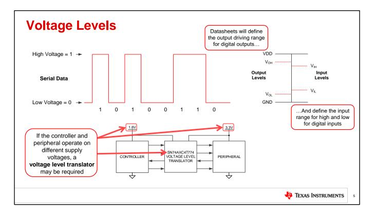
The lines between the controller and the peripheral device are driven to one of two voltage levels. If the voltage is near zero, then the line is decoded as a digital zero. If the voltage is near the digital supply, then the line is decoded as a digital one.
