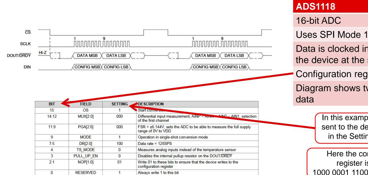
Data is clocked in and out of the device at the same time Configuration register is 16 bits
