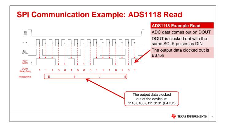
At the same time, the ADC data is clocked out of the ADS1118. Here, a random output data word is clocked out of the device. Looking at the DOUT line, the binary output is read as E475 in hexadecimal.
