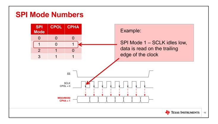
Combinations of CPOL and CPHA allow for four modes of operation of SPI. The table in this slide shows SPI modes 0 through 3. Each defines a different clock polarity and phase for SPI communication. Note that different manufacturers of SPI devices and microcontrollers may have different definitions of SPI mode numbers. Consult the datasheets for both the controller and peripherals to determine the clock polarity and phase information.
