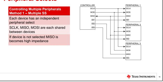
SPI can be used to communicate with multiple devices. This can be done in two different ways.
