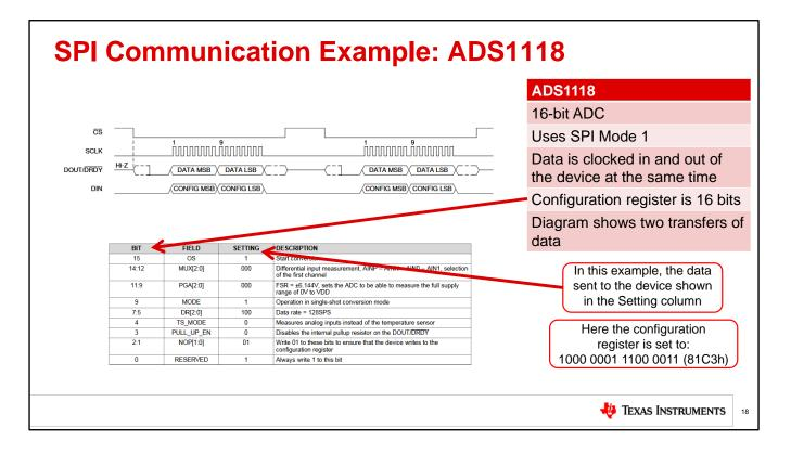
Here is an example of SPI data communication. This comes from the communication of the ADS1118 precision ADC.
