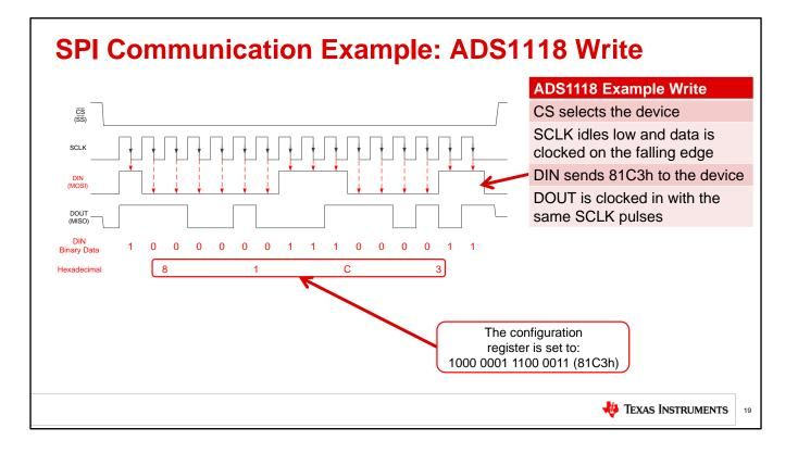
Continuing with the example, this is the 16-bit data transmission cycle for the ADS1118 showing the SPI lines. Again, the SCLK idles low, and data is transmitted at the falling edge of SCLK. The write to the device is done on the MOSI, or on this device, the pin is labeled as DIN. The configuration register is set to 81C3 in hexadecimal.
