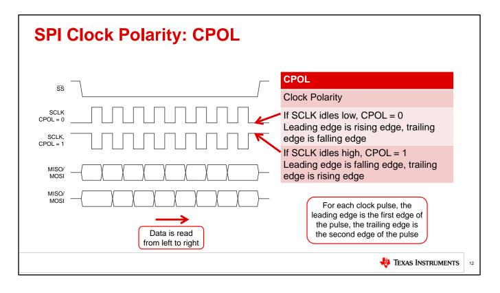
As previously mentioned, data from the controller and peripheral may be read on either the rising or falling edge of SCLK. Additionally, the clock polarity is important in defining the leading and trailing edges on which data is clocked in and out of the device. This enables several modes of SPI communication. There are two parameters used to determine modes of operation.
