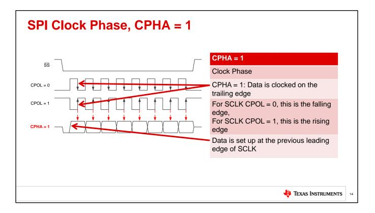
For CPHA equal to one, the data is captured on the trailing edge of SCLK. In both clock phase modes, data is set up on the previous clock edge.
