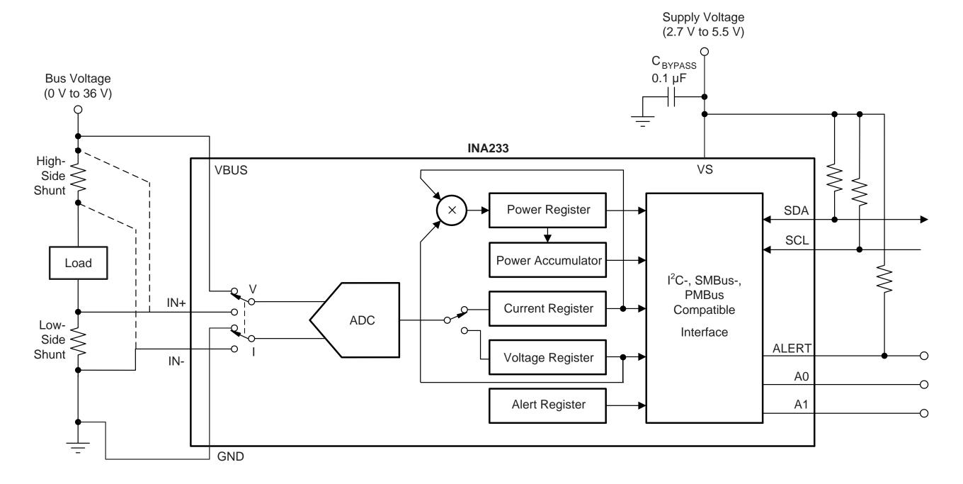
Digital power monitors are current sensing devices that measure both shunt voltage and bus voltage. A programmable calibration register, combined with an internal multiplier, also enables direct readouts of load current and power consumption.
