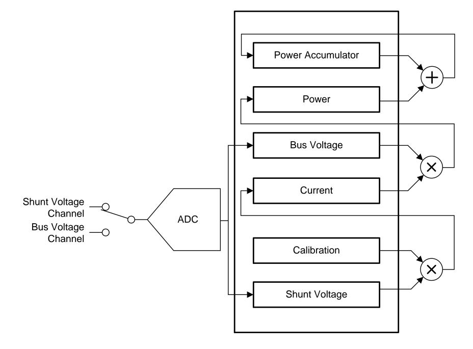
Let's take a closer look at the register structure of the digital power monitors. The shunt voltage, bus voltage, current, and power registers are all read only registers, while calibration register is a read/write register. There is no programming needed if you only require shunt and bus voltage measurements, and do not need direct current and power readouts.
