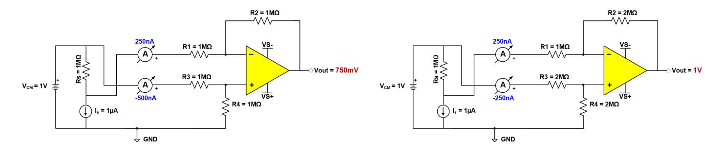
Differential input impedance: Rdiff = R1 + R3 Rdiff = Rs + R1 + R3 =  $3M\Omega$ Rdiff- = Rs + R1 =  $2M\Omega$ Rdiff+ = R3 =  $1M\Omega$ Common mode input impedance: Rcm+ and Rcm- = (R3+R4)||(R1+R2+Rs)
