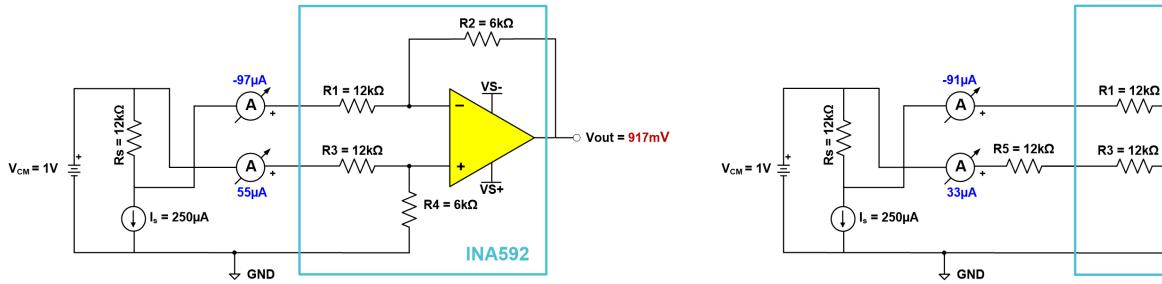
Differential input impedance:  $Rdiff = Rs + R1 + R3 = 36k\Omega$  $Rdiff = Rs + R1 = 24k\Omega$  $Rdiff + = R3 = 12k\Omega$ Common mode input impedance: Rcm+ and Rcm = (R3+R4)||(R1+R2+Rs)|| $Rcm = 11.25k\Omega$
