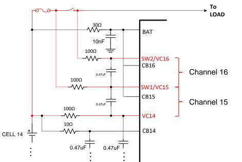
• Channels 16/15 can be used to diagnose the state of fuse and switch
