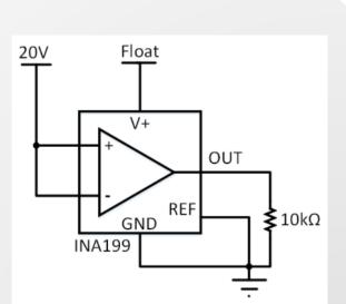
Vsupply = floating, (10 M $\Omega$  probe) Vout is gnd through 10 k $\Omega$
