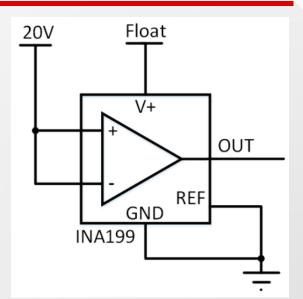
Vsupply = floating Vout and Vsupply measured (10 M $\Omega$  probe)
