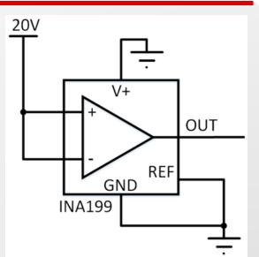
Vsupply = GND Vout and Vsupply measured (10 M $\Omega$  probe)
