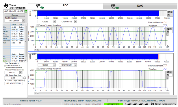
Figure 7-11. 200-MHz, Sine-Wave (Channel A) and 40-MHz, Square-Wave (Channel B) Time Domain for 5-GSPS, Single-Channel Oscilloscope
