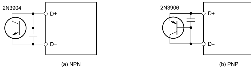
Figure 7-6. Remote Temperature Sensor Using Transistor
