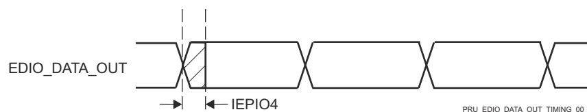
Figure 6-76. PRU-ICSS IEP Digital IOs Timing Requirements
