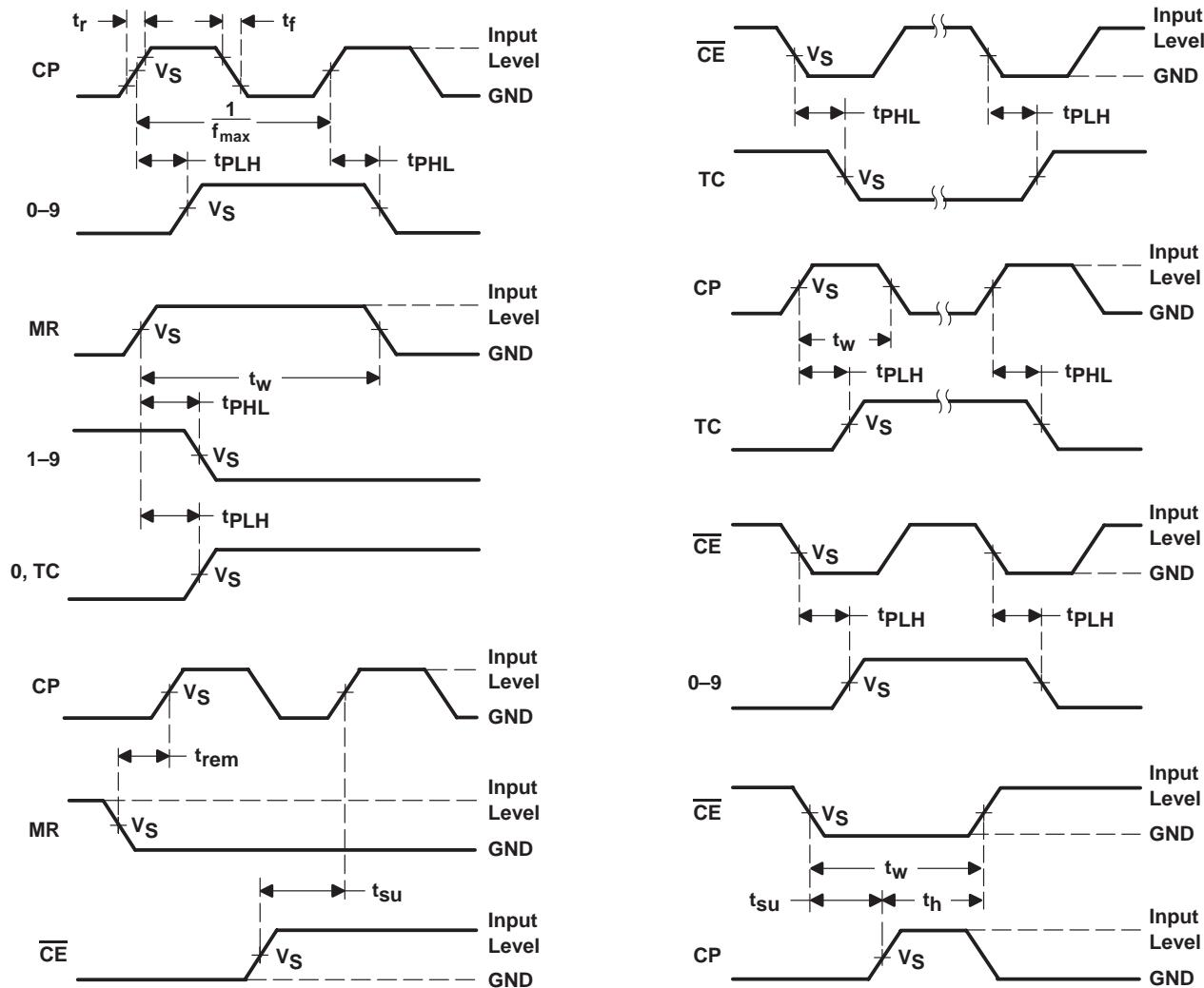
**Figure 2. Voltage Waveforms**
