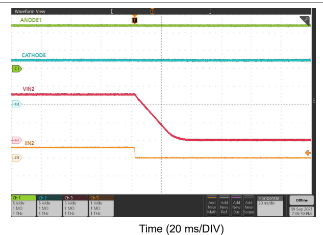
Figure 9-18. ORing - V_{IN2} Failure and Switch Over to V_{IN1}
