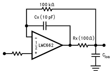
**Figure 6-3. Rx, Cx Improve Capacitive Load Tolerance**
