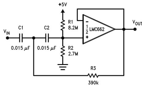
$f_c = 10\text{Hz}$ ,  $d = 0.895$ , gain = 1, 2dB pass-band ripple
