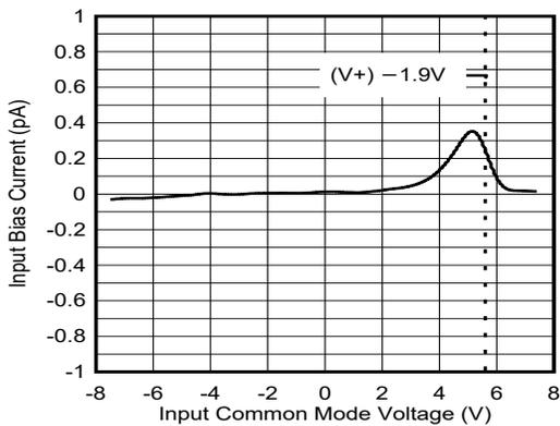
Figure 5-5. Input Bias Current vs Input Common-Mode Voltage
