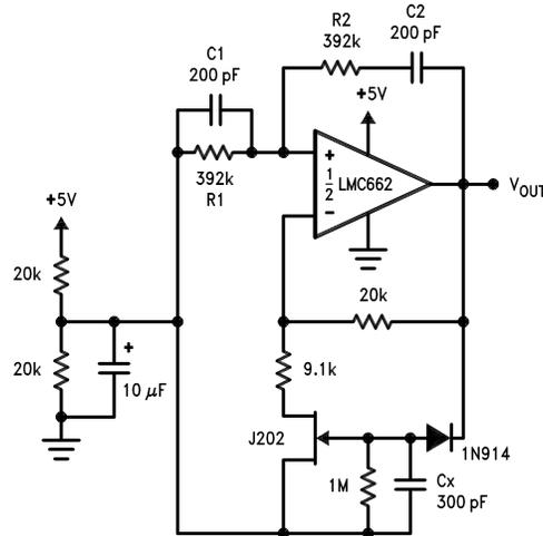
Oscillator frequency is determined by R1, R2, C1, and C2:
