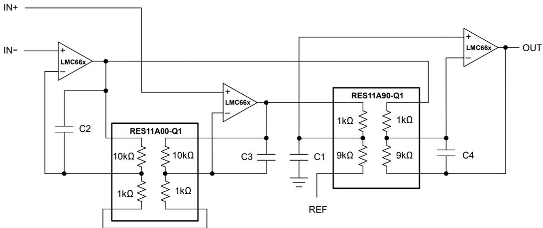
**Figure 6-8. Improved Instrumentation Amplifier With the RES11A**
