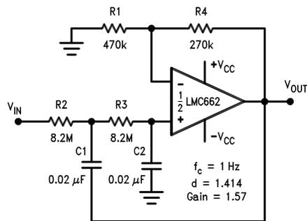
**Figure 6-14. 1Hz Low Pass Filter
