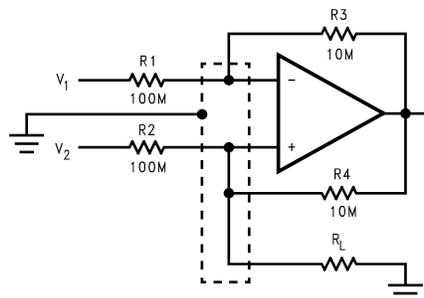
**Figure 6-20. Guard Ring Connections: Howland Current Pump**
