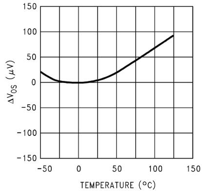
Figure 5-2. Offset Voltage
