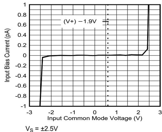
Figure 5-6. Input Bias Current vs Input Common-Mode Voltage
