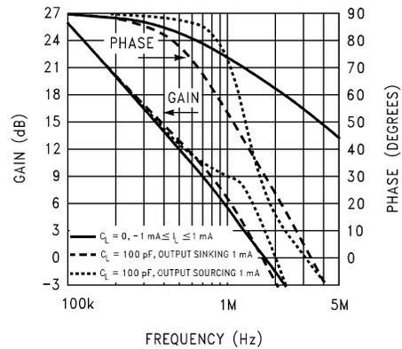
**Figure 5-12. Frequency Response vs Capacitive Load**
