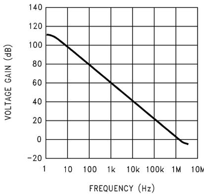
**Figure 5-11. Open-Loop Frequency Response**
