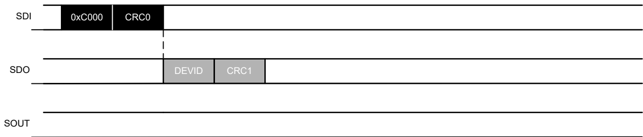
Figure 7-19. Example of REG_RD_CRC command
