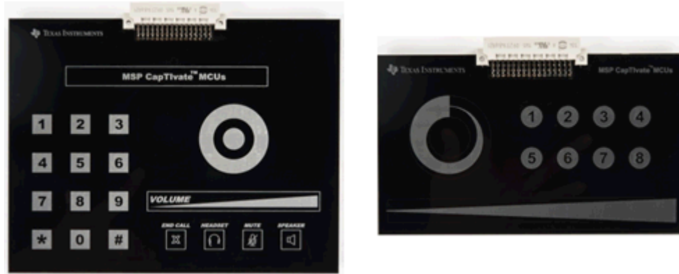
Figure 10-6. CAPTIVATE-PHONE and CAPTIVATE-BSWP Panels
