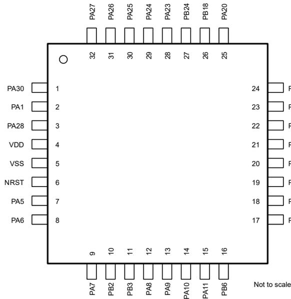
**Figure 6-5. 32-pin VFC (LQFP)**
