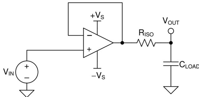
**Figure 7-2. Unity-Gain Buffer With  $R_{ISO}$  Stability Compensation**
