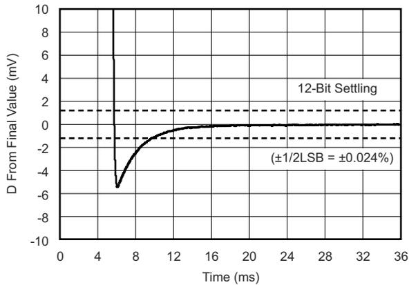
**Figure 5-33. Large-Signal Settling Time (10-V Negative Step)**
