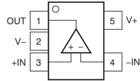
**Figure 4-2. OPA171 DBV Package: 5-Pin SOT-23 (Top View)**
