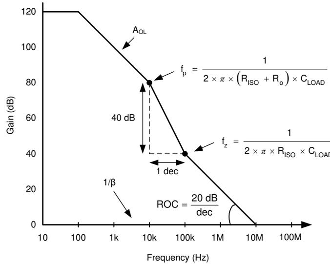
**Figure 7-3. Unity-Gain Amplifier With  $R_{ISO}$  Compensation**
