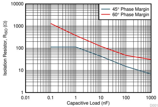
Figure 7-6. R<sub>ISO</sub> vs C<sub>LOAD</sub>
