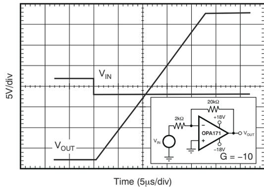
Figure 5-27. Negative Overload Recovery
