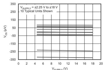
Offset Voltage vs Power Supply
