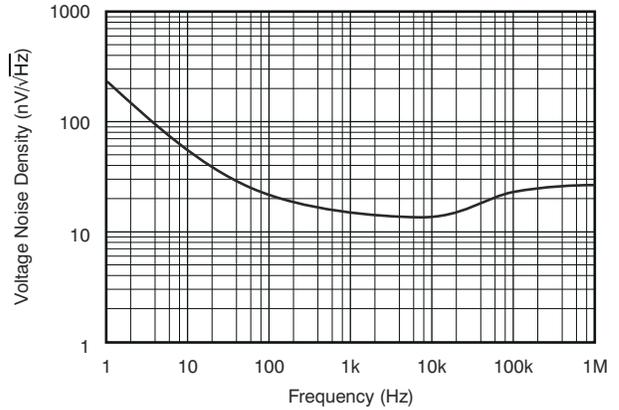
**Figure 5-14. Input Voltage Noise Spectral Density vs Frequency**
