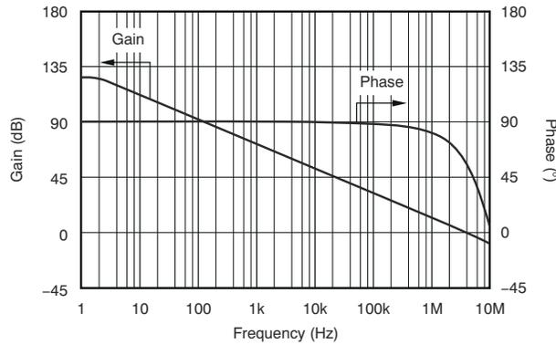
**Figure 5-19. Open-Loop Gain and Phase vs Frequency**
