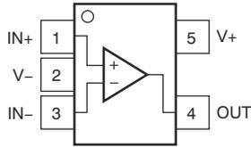
**Figure 4-1. OPA171 DRL Package: 5-Pin SOT-553 (Top View)**
