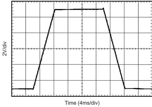
**Figure 5-31. Large-Signal Step Response**
