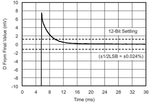
**Figure 5-32. Large-Signal Settling Time (10-V Positive Step)**
