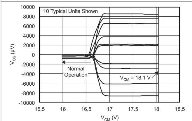
**Figure 5-5. Offset Voltage vs Common-Mode Voltage (Upper Stage)**
