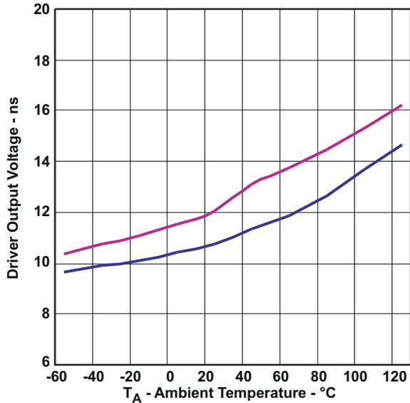
**Figure 6-5. Driver Differential Delay Times vs Free-Air Temperature**
