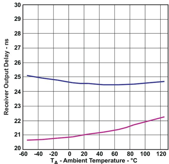
**Figure 6-12. Receiver Propagation DELAY T<sub>I</sub> vs Free-Air Temperature**
