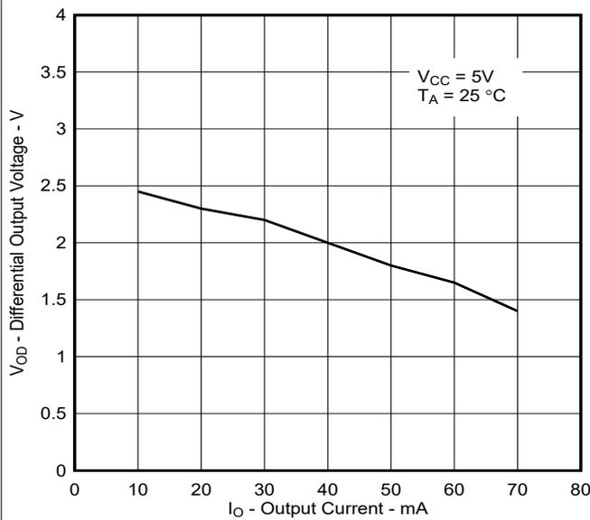
**Figure 6-3. Driver Differential Output Voltage vs Output Current**
