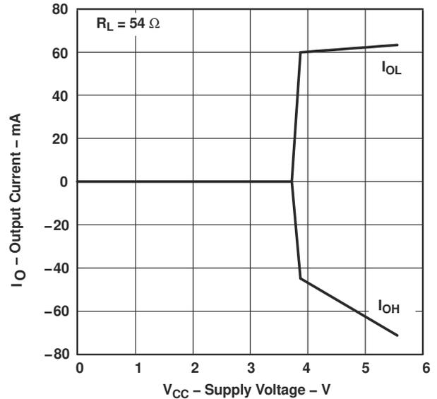
**Figure 6-6. Driver Output Current vs Supply Voltage**
