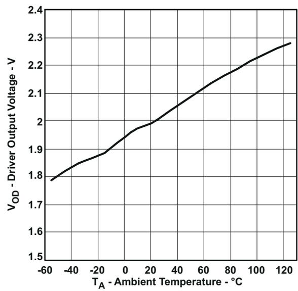
**Figure 6-4. Driver Differential Output Voltage vs Free-Air Temperature**
