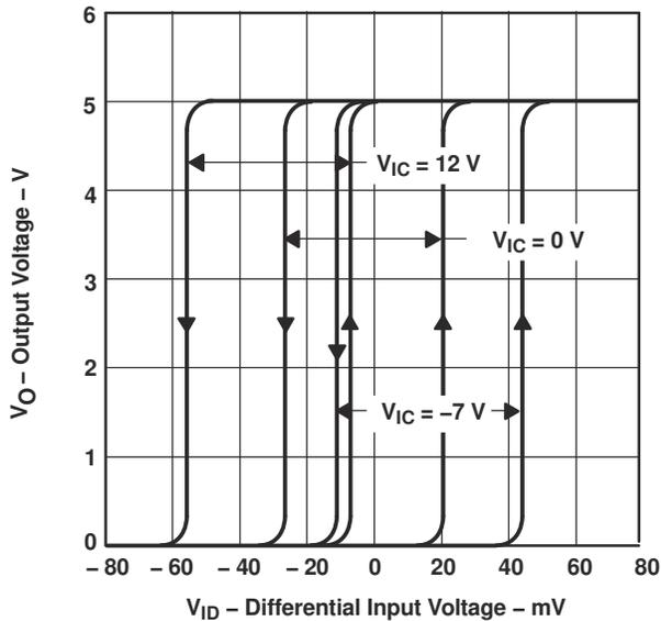
**Figure 6-9. Receiver Output Voltage vs Differential Input Voltage**
