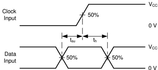
**Figure 6-3. Voltage Waveforms, Setup and Hold Times**
