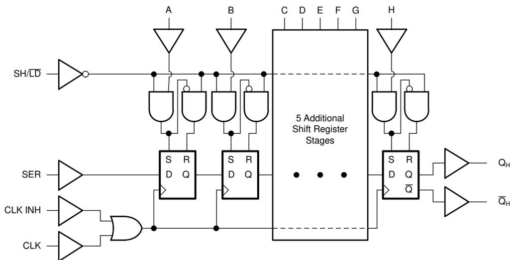
Figure 7-1. Logic Diagram (Positive Logic) for SN74AC165
