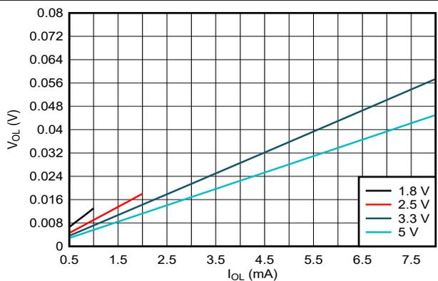
Figure 5-6. Output Voltage vs Current in LOW State
