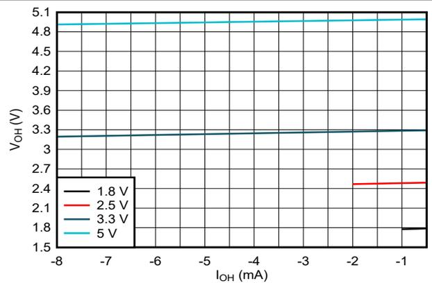
Figure 5-5. Output Voltage vs Current in HIGH State
