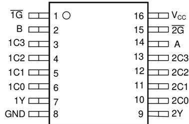
**PW Package, 16-Pin TSSOP (Top View)**
