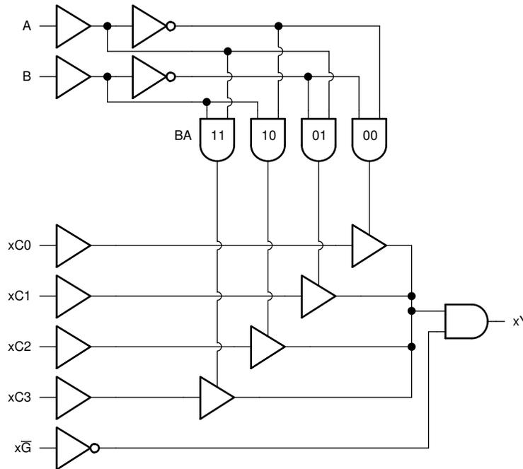
Figure 7-1. Logic Diagram (Positive Logic) for SN74ACT153
