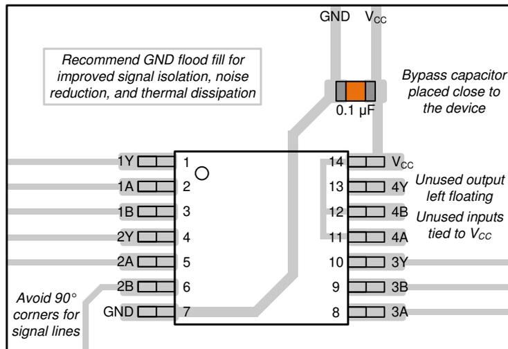
**Figure 8-3. Example Layout for the SN74LV4T02-EP**
