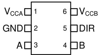
Figure 5-3. DRL Package Preview 6-Pin SOT Top View
