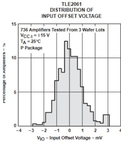
Figure 5-1. TLE2061 Distribution of Input Offset Voltage
