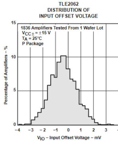
Figure 5-2. TLE2062 Distribution of Input Offset Voltage
