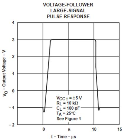
Figure 5-9. Voltage Follower Large Signal Pulse Response
