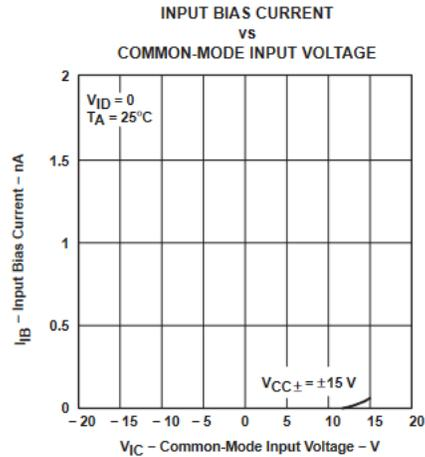
Figure 5-4. Input Bias Current vs Common Mode Input Voltage
