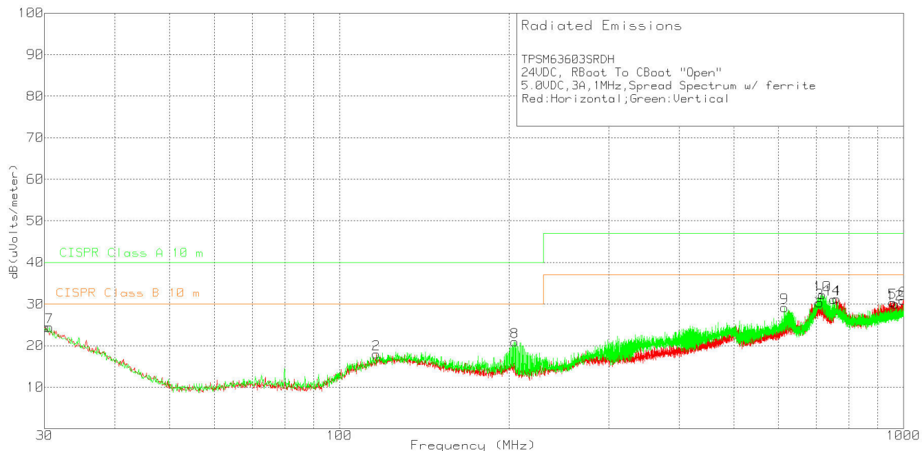
Figure 9-14. Radiated Emissions, 24-V Input, 5-V Output, 3-A Load, Spread Spectrum
