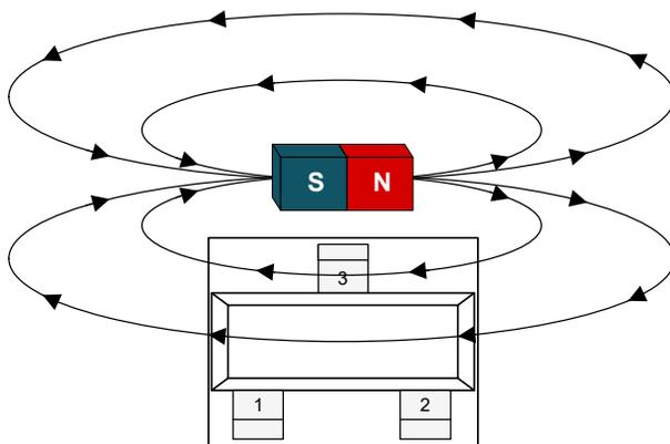
Figure 7-5. Positive Magnetic Flux Density: Magnet Offset
