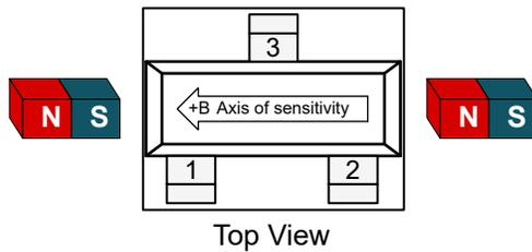
Figure 7-3. Positive Magnetic Flux Density
