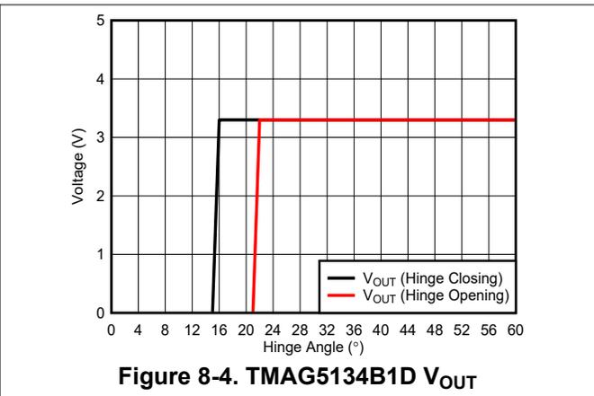
**Figure 8-4. TMAG5134B1D  $V_{OUT}$**
