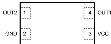
Figure 5-2. ZFC Package, 4-Pin X1LGA (Top View)
